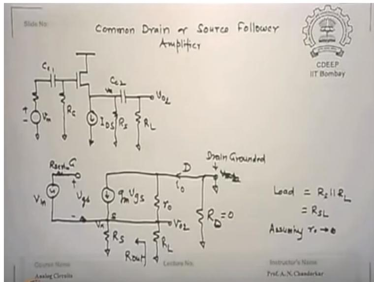
So this is why we still use these amplifiers then we also did something about the common drain or source follower essentially the difference between the last one and this is that this there is no drain resistance  $R_D$  is 0 in this case  $R_D$  is 0 that is why it is common drain it is going to the ground drain is going to the ground and the output is taken at the source itself output is taken at the source and this is that first resistance  $R_S$  this is additional load resistance.
