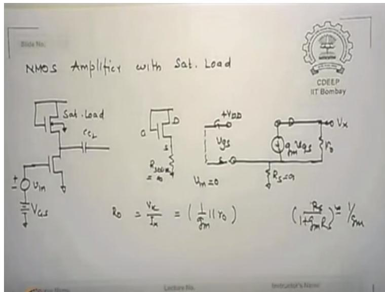
Before we quit this area quickly I will I will not solve all of it there are different kinds of load I say in the case of loss amplifiers one of the mass amplifier will have okay by the way this terminology you should use their input is connected that transistor is called driver okay and the resistance is replaced by a transistor that is called load.
