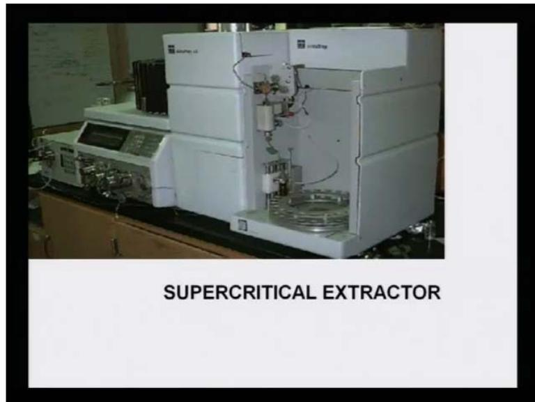
Now SUPERCritical EXTRACTOR: This is how it looks and there is this liquefied carbon dioxide, which is popularly used for the extraction of the colorant. Sometimes some entrainers are added as a solvent like ethyl acetate, to facilitate the solubility of the colorant. Now because of the rarefaction of carbon dioxide, and liquid fraction of carbon dioxide, it adds on property to the liquid carbon dioxide, to be a good solvent.
