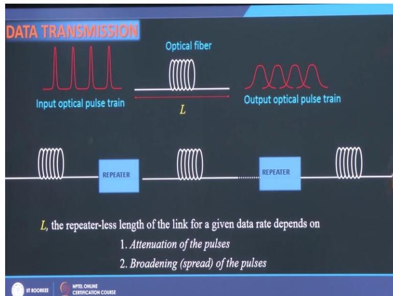
And when I send this pulse train through an optical fiber, then at the output end the shape of the pulses becomes something like this. What I notice here is the amplitude of these pulses the power level of these pulses it goes down, and at the same time the duration of pulses increases.
