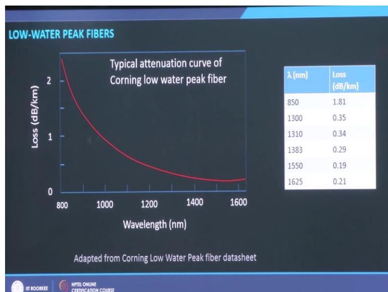
So, this is state of the art fiber from Corning glass works, which is low water peak fiber and I can see here that it is very smooth attenuation curve and it does not have any peaks and if I look at losses at various wavelengths, it is extremely small loss. So, you can see near 1380 nanometer wavelength, where we had very large water peak, now it has loss of only 0.29 dB per kilometer, at 1550 it has a loss of 0.19 dB per kilometer.
