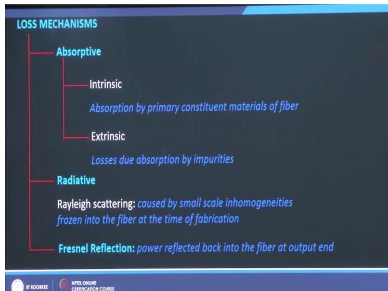
Now, what are the lost mechanisms in an optical fiber what causes loss?
