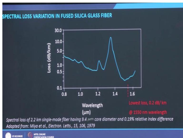
And if I look at the spectral loss variation in fused silica glass fiber it looks like this, this is the spectral loss of 2.2 kilometer single mode fiber with core diameter of 9.4 micrometer and about 0.2 percent relative index difference.
