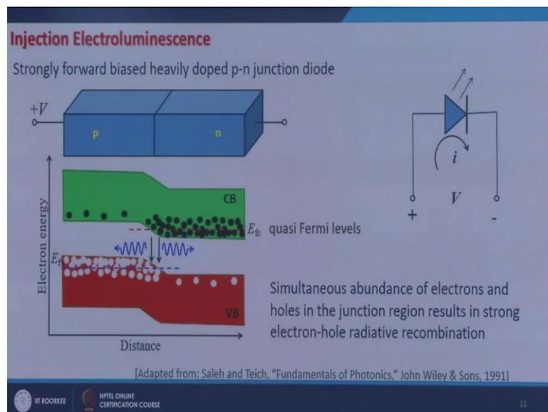
So, I explain this with the help of a strongly forward biased heavily doped  $p$ - $n$  junction diode. So, if this  $p$ - $n$  junction is heavily doped, then there are large number of electrons in the conduction band and large number of holes in the valence band such that this Fermi level goes even inside the conduction band and this Fermi level shifts to inside the valence band and these are known as quasi Fermi levels.
