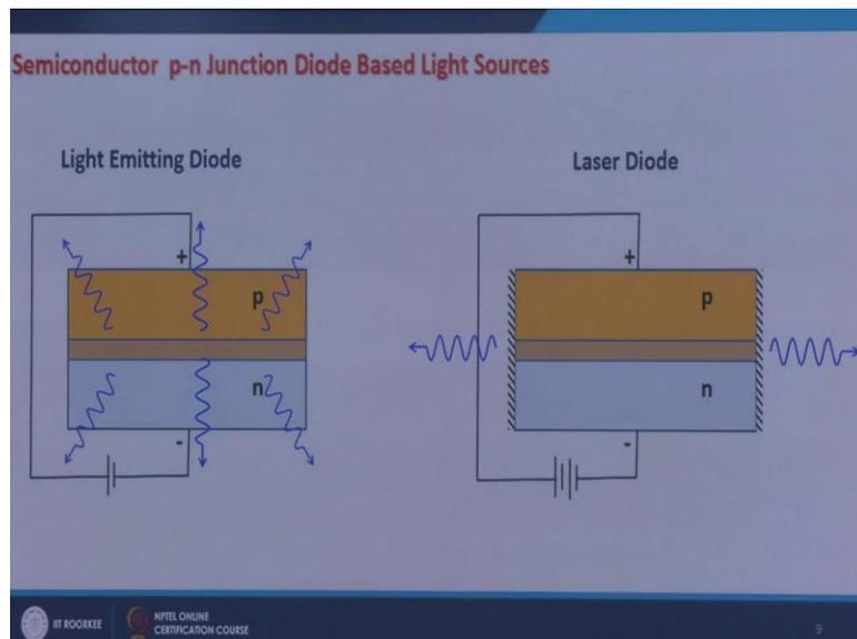
So, we have semiconductor  $p-n$  junction diode based light sources is light emitting diode where the light generation is via the process of spontaneous emission. So, what you do you forward bias a  $p-n$  junction diode by forward biasing it, you are basically injecting the
