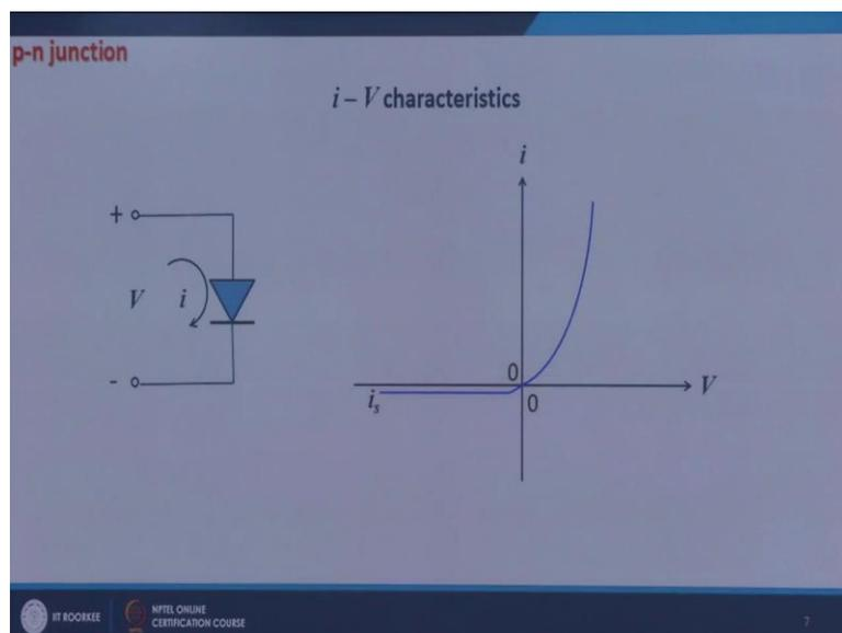
So, if you look at the  $i-V$  characteristics of a  $p-n$  junction. So, in forward bias if you increase the voltage the forward current will increase; however, if you apply the negative voltage and
