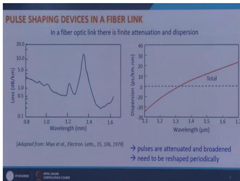
So, what happens when pulses travel through optical fiber? They get attenuated and they get dispersed. Typical attenuation curve; you know of an optical fiber is like this and a typical dispersion curve is like this. So, when these pulses are attenuated and dispersed then periodically we need to reshape the pulses.
