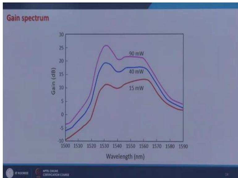
If you look at the gain at different wavelengths that is at the gain spectrum then it looks like this particular characteristic comes from the emission cross-section and absorption cross-section of the EDFA.
