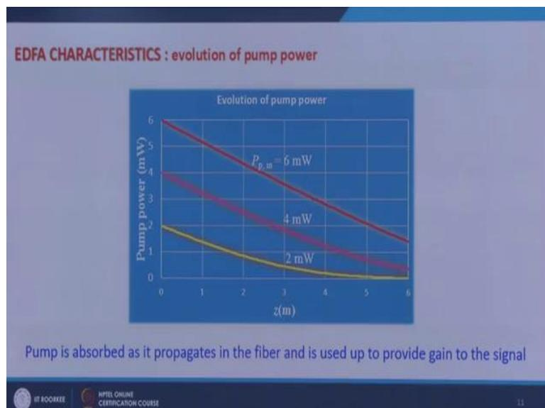
Let us look at typical characteristics of an erbium doped fiber amplifier here I show the evolution of pump power how the pump power varies with the distance in the fiber.
