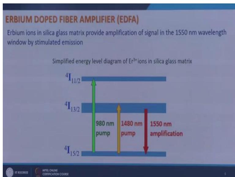
So, how do we amplify this signal in an optical fiber amplifier? We make use of erbium ions in silica glass matrix and do amplification by stimulated emission of radiation the principle which is involved in the laser itself.
