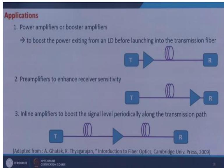
What are the applications? Applications of EDFA are in power amplifiers or booster amplifier what you can do before sending the signal into the transmission link fiber link you can first boost the signal using an amplifier then it is known as booster amplifier.
