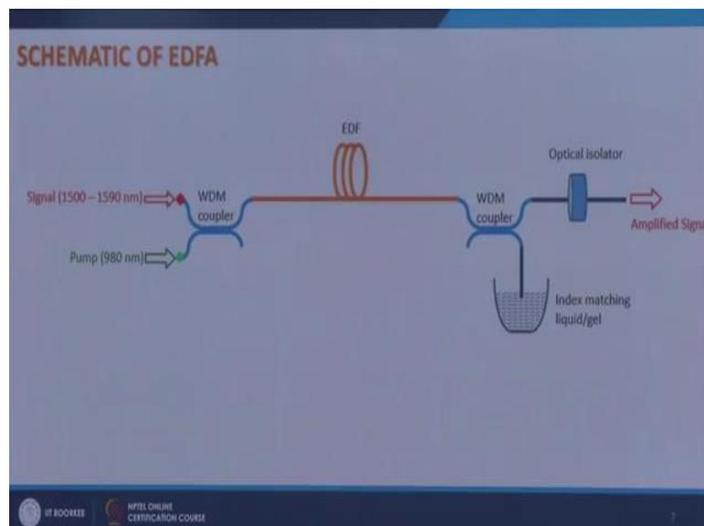
This is a schematic of an EDFA. So, you need to know what you want to do; you want to amplify signal which lies in this wavelength range with the aid of the pump which provides energy for amplification of signal and this pump is at 980 nm.
