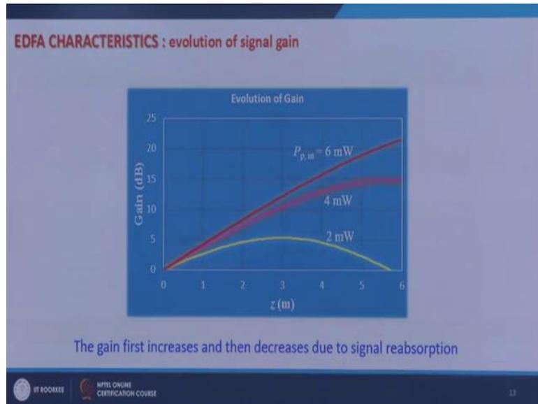
So, initially the pump is able to provide energy to the signal. So, your gain increases after that it gets almost saturated and then again it decreases because of signal re-absorption.
