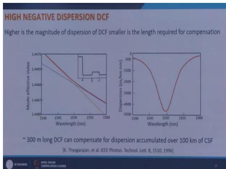
How do you achieve this kind of dispersion? There is a design which is given by Tyagarajan in 1996 where they have used this dual core fiber and this particular fiber gives you the effective index as a function of wavelength something like this which makes a turn which makes a turn somewhere here and the curvature changes here and because of the change in curvature at this point you will have very high value of the second derivative of an effective
