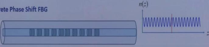
Phase shift opens a narrow transmission window within the stop band in the transmission spectrum
