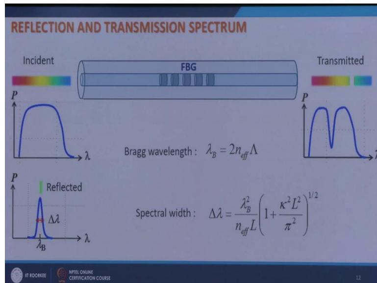
Let us now look at reflection and transmission spectrum of the grating. If I incident this spectrum which is broadband spectrum, then out of all these wavelengths only one wavelength which satisfies the condition  $2 n_{\text{effective}} \Lambda = \lambda_B$ , that wavelength will be reflected and all the other wavelengths will pass through. So, in the transmitted spectrum this wavelength  $\lambda_B$  would be missing and in the reflection spectrum this wavelength will appear.
