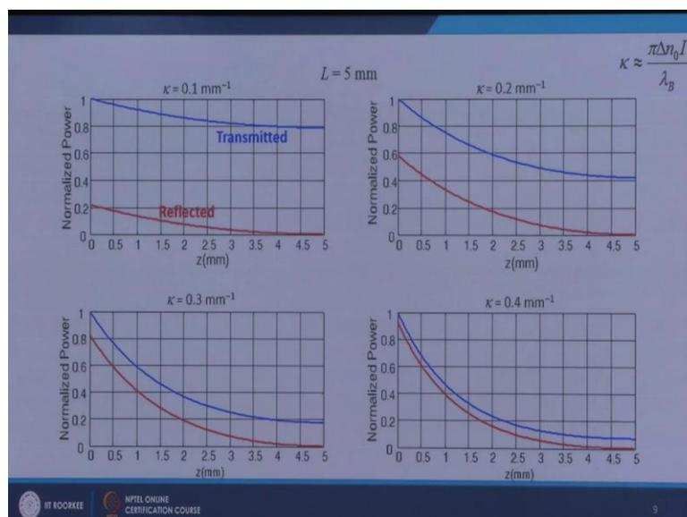
Here, I show how the power in the transmitted and reflected modes vary as a function of  $z$ , what is the evolution of power in the forward and backward propagating modes for different values of  $\kappa$ . For a given grating length  $L$  is equal to let us say 5 millimeters I can see that when  $\kappa$  is the small value say 0.1 milliliter inverse, then ~~then~~ even at  $L$  is equal to 5. I
