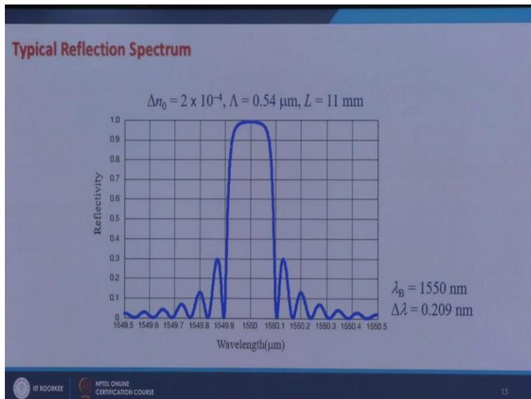
This is typical reflection spectrum for  $\Delta n_0$  is equal to  $2 \times 10^{-4}$ , grating period about 0.54 micro meter and  $L$  is equal to 11 millimeter for a typical single mode fiber.
