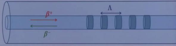
Grating acts as a perturbation which enables coupling of light between the forward and backward propagating modes
