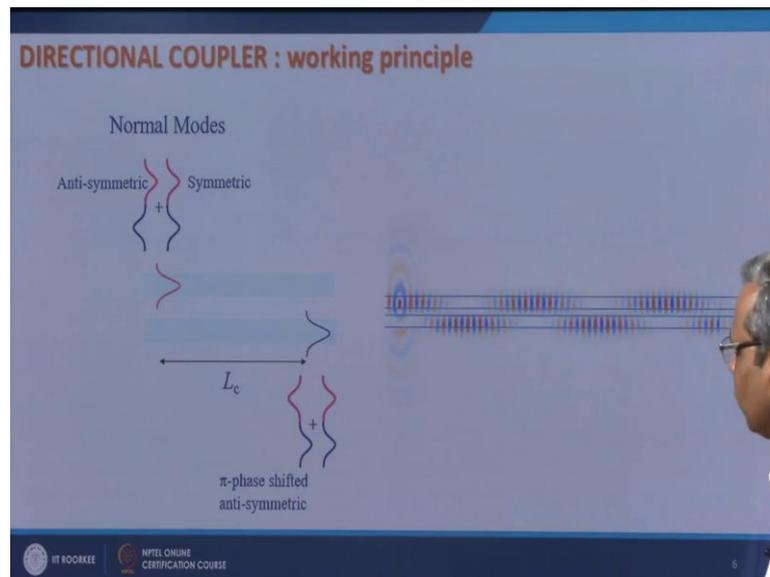
So, exciting core 1 with an appropriate field pattern is equivalent to exciting symmetric and antisymmetric modes equally.
