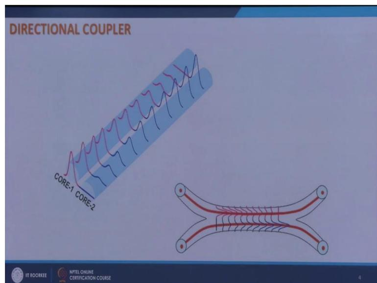
Then as this light propagates through optical fiber this composite system then, then there is a redistribution of power between the 2 cores and after a certain length all the power will come out of the other core. So, there is a switching of power from core 1 to core 2. So, if I look it look at it as a 4 port device then this is port 1, port 2, port 3, port 4, and if I launch light in core 1 then light may come out of core 2 in the output end.
