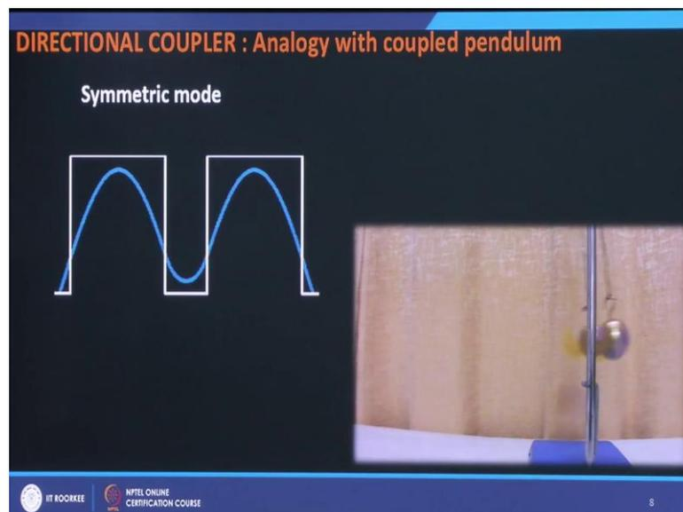
This color is changing it indicates that the power is going along the length of fiber along the length of the directional coupler. So, this is the field distribution at different lengths of the fiber as the color changes it means the length is changing. So, I am changing the length, but it retains its shape. So, the symmetric mode it retains its shape, and this is equivalent to the couple pendulum when these two bobs are moving together. And they keep on doing like this.
