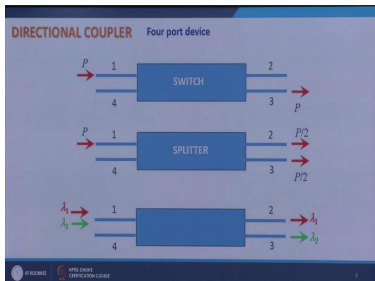
A very basic components and very important component using optical fiber is directional coupler. What is the directional coupler? It is essentially a 4 port device. So, we have a fiber here a fiber coming out here, a fiber coming out here, and fiber going inside here. What we can have using this well if we launch power  $P$  in port 1, depending upon the
