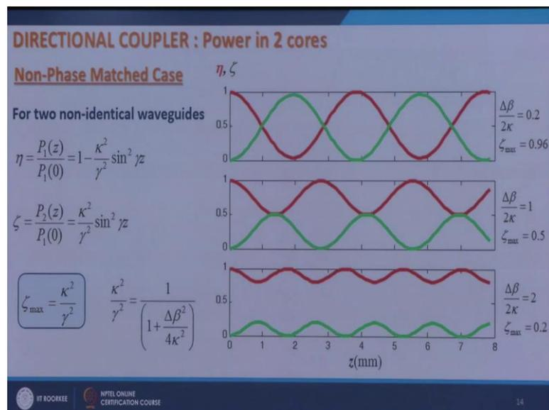
And the fraction of power that appears in core 2 is  $\zeta = \frac{P_2(z)}{P_1(0)} = \frac{\kappa^2}{\gamma^2} \sin^2 \gamma z .$
