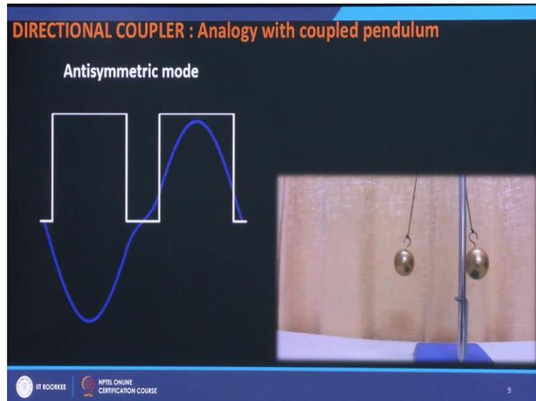
So, this is symmetric state of the couple pendulum this is symmetric normal mode of the directional coupler. I can have antisymmetric when I displace one on this direction another in this direction. So, they will keep on doing like this. And this is how this field is also retaining its shape when it propagates along the length of the fiber.
