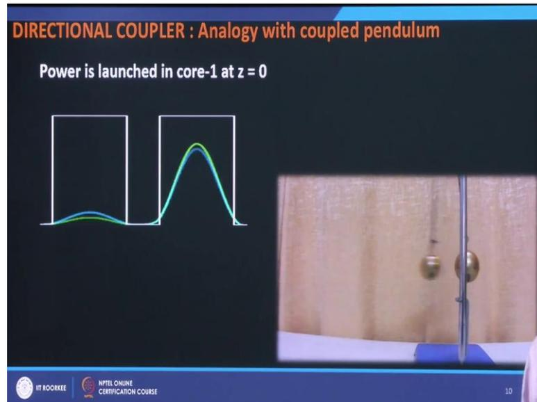
So, there is periodic exchange of energy between the two bobs. Similarly, here if I have all the powers here at  $z = 0$ , then as the power propagates along the length of the system then the power periodically transfers from one core to another core. So, there is periodic coupling power couples back and forth between the 2 cores. So, this is how by just a simple analogy of a couple pendulum we can understand the phenomenon of coupling of power from one core to another core.
