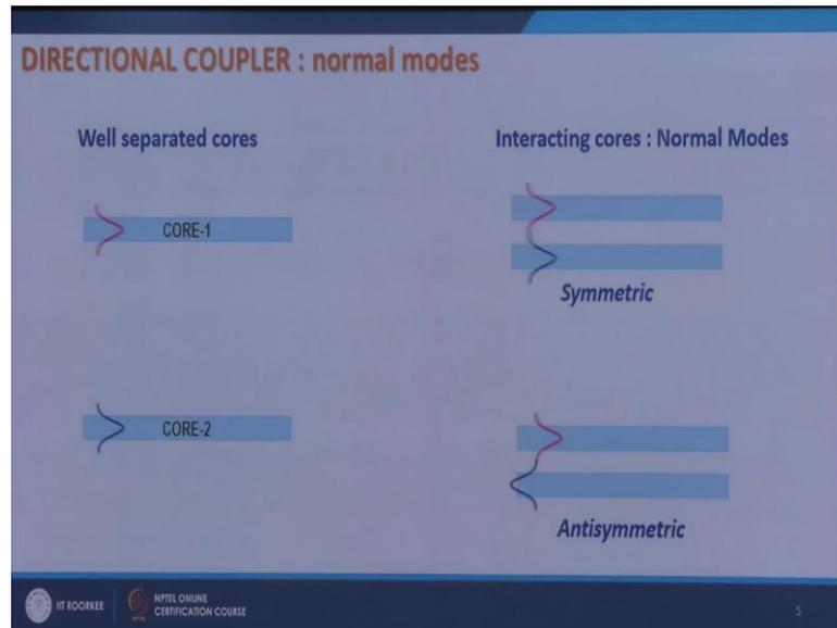
So, if I have 2 fibers which are very well separated and these are single mode fibers, then this fiber supports this mode this fiber supports this mode. And propagation of light in this fiber is not affected by the propagation of light in this fiber, because they are very well separated. But if I bring them closer then what may happen that now this is core 1.
