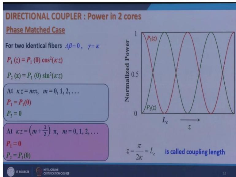
It depends on the fiber parameters, the core separation and the wavelength. So, if I have 2 identical fibers then  $\beta_1 = \beta_2, \Delta\beta=0$ . And if  $\Delta\beta=0$  then  $\gamma=\kappa$ . If you go back to this expression let me retain this expression in on the board that that  $P_1(z)=P_1(0)\cos^2 \kappa z$  and  $P_2(z)=P_1(0)\sin^2 \kappa z$ .
