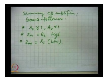
In summary of CD, common drain amplifier, which is also known as source follower, source follower, here the gain is close to 1, but actually, it is less than 1 and input impedance very high, R G and output impedance, R s, low and it is used for buffer purposes.
