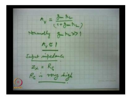
g m into r L, normally is much higher than 1, that is, A v we have obtained as g m r L 1 plus g m r L. Normally, usually g m into r L is very large as compared to 1, so 1 can be dropped, then A v will be very close to unity. When A v is 1, that implies, that there is no voltage gain, there is no voltage gain, it, it is, whatever is the input, same appears at the output, but there will be some power gain. Now, so this is this.
