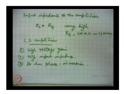
And then, the input impedance, input impedance of the amplifier; input impedance of the amplifier. We can see from, for example, from this model that input impedance, if we measure at the input terminals between gate and source, this will come out to be equal to R G and R G is very high. So, input impedance Z i, this is equal to R G, this is very high. Normally, R G will have range, 100 kilo ohms to 1000 or more kilo ohms. So, input impedance is very high.
