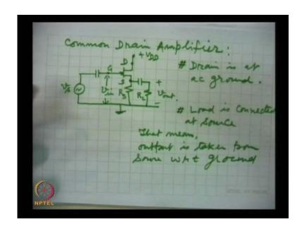
Then, we go for the next amplifier, that is, common drain amplifier, common drain amplifier. Let us first draw the circuit.
