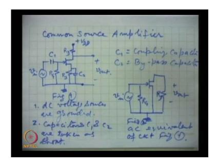
First, we take common source amplifier, common source amplifier, which for example, the JFET can be drawn like this.
