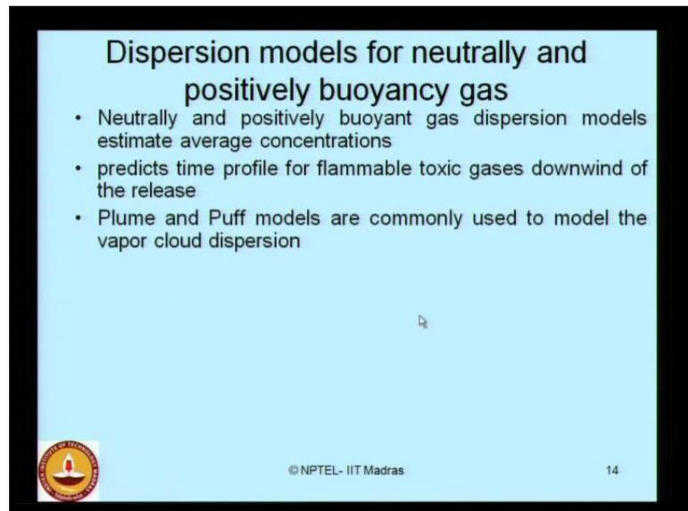
**Dispersion models for neutrally and positively buoyancy gas**
