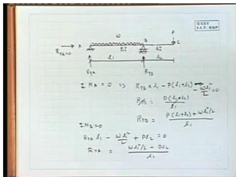
So, the beam is like this ABC; at A there is one support - simple support; B another simple support; C is free. So, free end, there is a load P. A to B it is fully loaded with some uniformly distributed load; intensity is omega. AB length say it is defined as  $l_1$ ; BC it is defined as  $l_2$ . For simplicity, entire beam having a identical cross section EI. Now, for that beam we are interested to find out the form, say, for the deflected shape of the beam.
