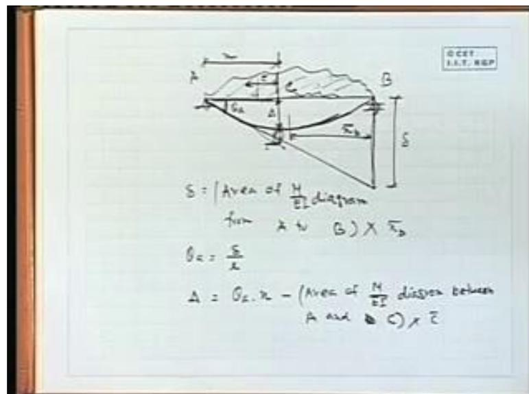
Now, how will we handle a case of a simply supported type of problem? Now, it will undergo some deformation like this. It may be some loading. Now, if you are interested to find the slope at the supported end or deflection at the middle of the span or some intermediate point, just like cantilever, we cannot get it; but here, more or less we will follow that type of procedure.
