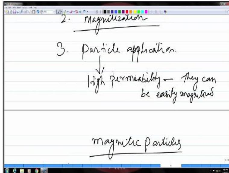
Any particle which have high magnetic permeability, like iron particle, for example, can be used for doing magnetic particle testing.
