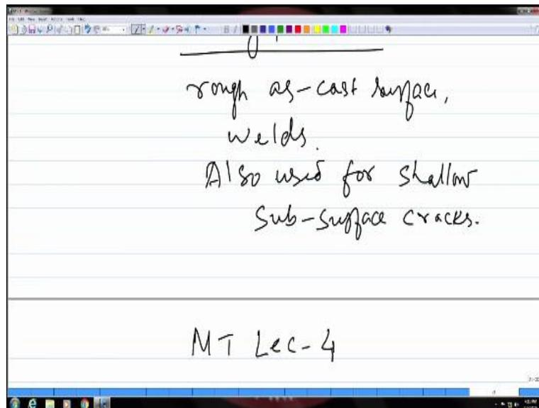
And the dry powder is also useful for doing shallow subsurface cracks, apart from the surface cracks. This dry powder can also be used for doing some subsurface inspection. So, let us continue today.
