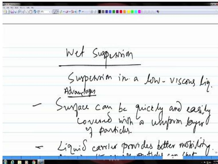
And this wet suspension has certain advantages over the dry powder and in certain cases, where the wet suspension cannot be used, like a rough surface, in those cases a dry powder is recommended.
