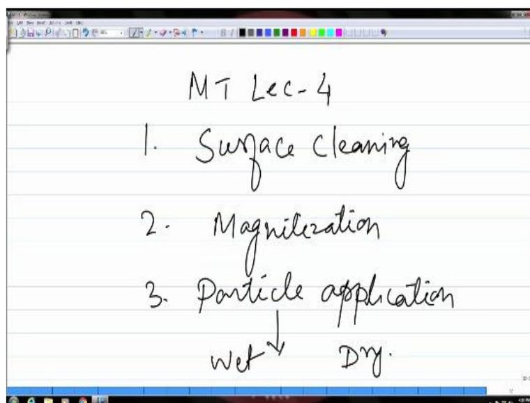
We have, so far, covered these three steps, surface cleaning, then magnetizing and once the part is magnetized, you apply the particles and in this, we saw there are two types, wet and dry, which are used depending on the surface condition.
