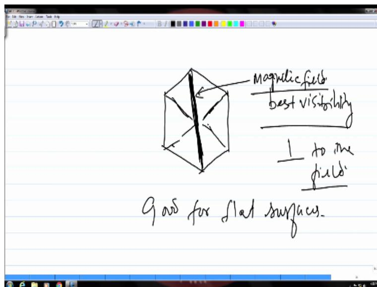
And then, these slots you have, so when you see the other surface, the other side of this, it is completely flat. So, this is what you will see on the other side of this pie gage. There is no slot or anything on this surface. So, you keep this offside down, that means a slotted side will be down and then magnetize. Once you magnetize and then start applying the particles, you will see, some of those slots being indicated on the other side, like this you would see.
