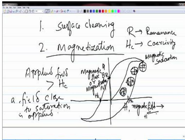
So, this is what, we discussed in the previous class, which was about magnetizing the surface and then, we saw that in terms of the magnetic field, which is needed to magnetize the part, you need
