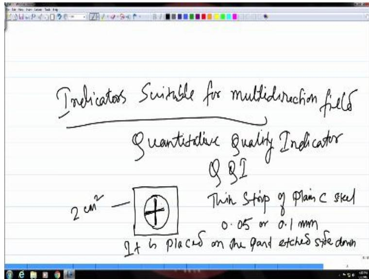
So, in those cases you need the indicators which are suitable for multiple directions or multidirectional fields. And this kind of indicators which are used for multi directional fields are also sometimes referred as quantitative quality indicators or QQI, in short. So, that means, in this case, you need some feature on the indicator which can indicate the direction of the field in different directions.
