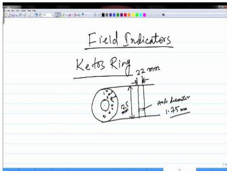
So, while doing the test, you do not know, what actually is the magnitude of the field, which is being applied? So, in that case, you need some indicators which will indicate whether the field is optimum or whether the field is enough or not, in a qualitative manners.
