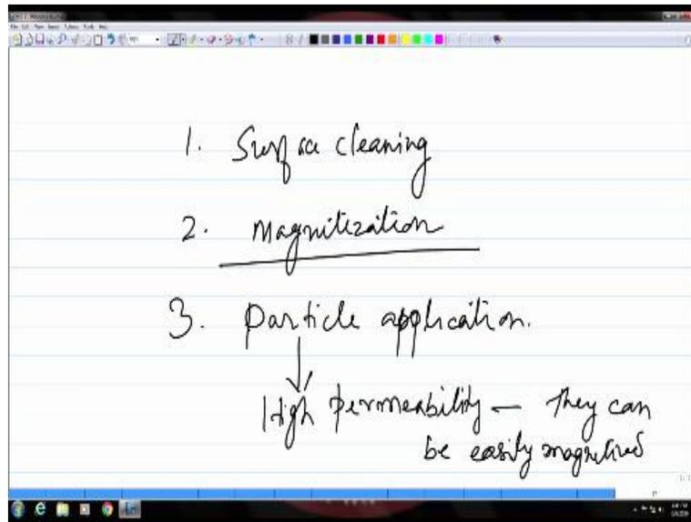
So, let us see, in what stage we are for this particular technique on magnetic particle testing. So, the first one was surface cleaning, then, magnetizing and in this magnetization, we have seen different methods and we have also learned about the theory of magnetism, which is needed in this case and then you saw how a field indicator can indicate the magnitude and the direction of the field, which is being applied to magnetize the part.
