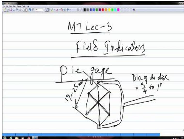
So, let us continue on that. So, one of the field indicators we have seen but we have couple of more to talk about. The next one that we have is called a pie gage and this is again a small coin, which is made of a highly permeable magnetic material and this coin can be divided into six or eight parts. So, it can be a hexagon or an octagon. So, this is as big as one rupee coin made of a highly permeable, magnetic material.
