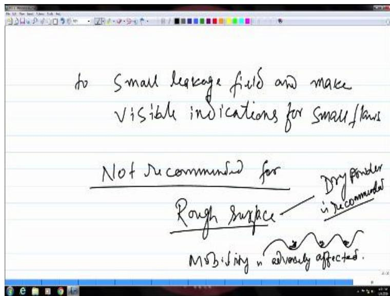
So, these are some advantages that you have, when you use a wet suspension rather than dry particles. But in case of certain scenarios, these wet suspension or wet particles are not recommended for a rough surface. So, if you have high surface roughness, like, you have lot of undulation on the surface, so then, this kind of wet particles are not recommended because in that case, in these valleys that you have, these particles will tend to segregate along these valleys.
