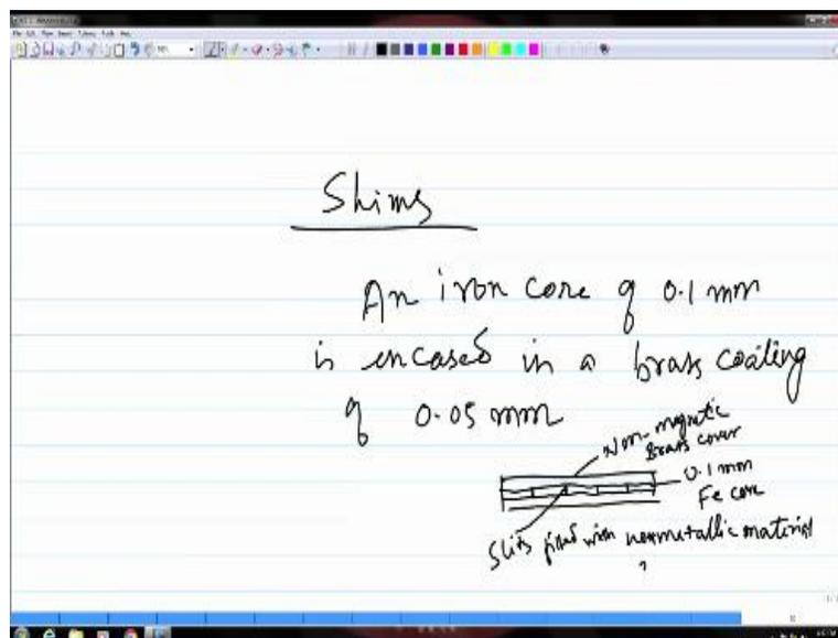
Then, you have something called, this is again part of the same similar kind of field indicators, and these are known, as shims. So, it could be like a thin strip of magnetic material again, which is covered by a non-magnetic material. For example, an iron core of 0.1mm is encased in a brass coating. So, this ferromagnetic iron core is coated by a thin brass casing. So, it is the magnetic core is coated, by a non-magnetic material like brass, of around 0.05 mm thick.
