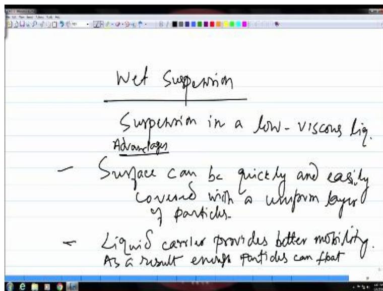
Suspension in a low viscous liquid, so, some petroleum liquid, for example, kerosene can be used because it satisfies the property requirements like low viscosity, uniformity, wetting and so on. So, that kind of petroleum liquid can be used to make the suspension and it has many advantages over dry particles, for example, if you look at the advantages; the surface can be quickly and easily covered because the liquid acts as the carrier and provides mobility to the particles.
