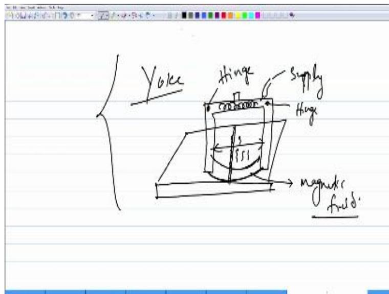
And then, we talked about this also, a U-shaped electromagnet, which is known as a yoke, that can also be used to magnetize the part and in this case, the direction of the magnetic lines, the magnetic lines of force, are across this. If you connect these two legs, so, along this line is the direction of the magnetic field. So, that means cracks, which are lying like this, perpendicular to this field, will have the best visibility.
