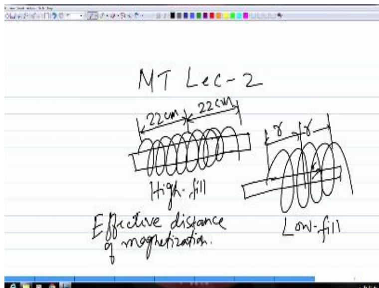
Similarly, when you are using this kind of coil, depending on whether the diameter of this coil is tightly filled by the part or the part diameter is much smaller compared to the diameter of the coil
