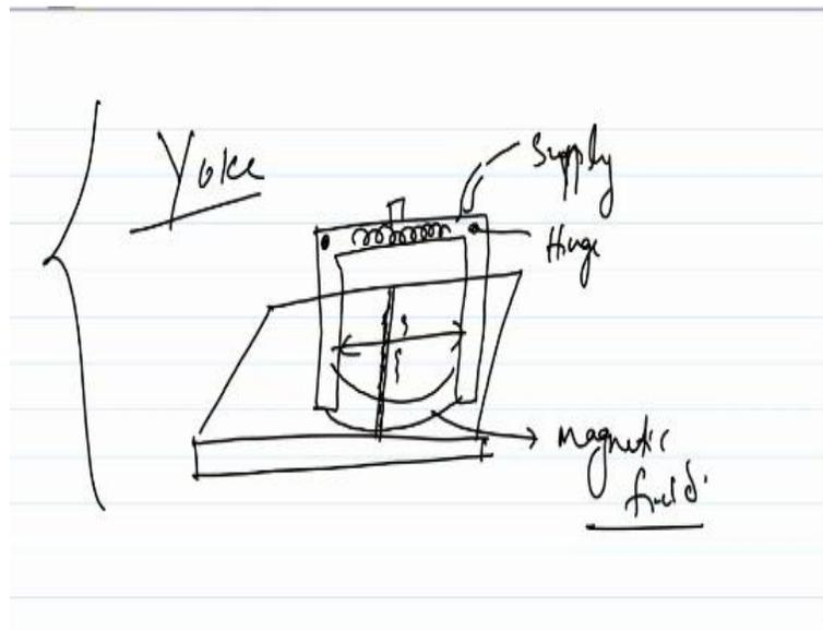
So, inside this, you essentially have a coil, which carries the current and then you can connect it to a power supply and you might have a switch, to switch on the current and the moment you switch on, the current, it will start the magnetic current and create the magnetic field across this. So, let us say you want to inspect this weld. So, these are the two plates, which are welded.
