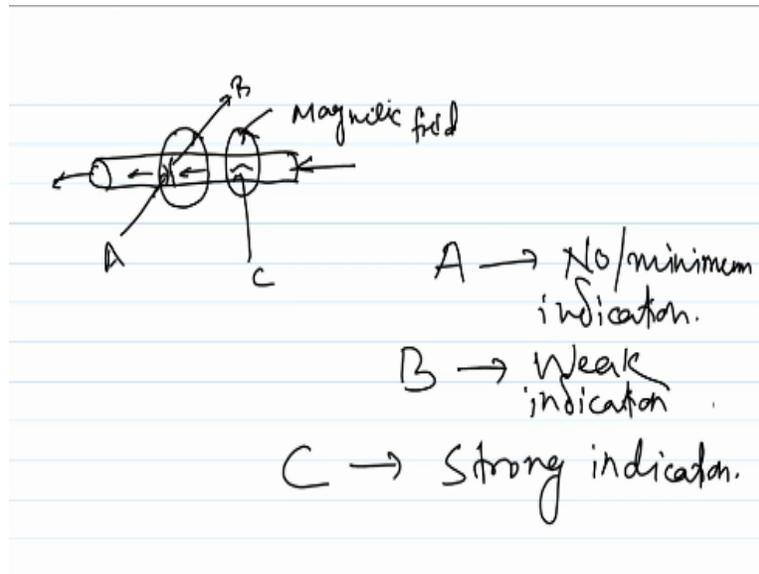
For example, if you have the current and the magnetic field like this and let us say you have a very regular discontinuity like this, which is parallel to the direction of the magnetic field's. So, this is your magnetic field, as I showed in the previous diagram also, and you have another, which is not very regular, the crack is little, you know, uneven. This first one, let us call that as A, this one as B.
