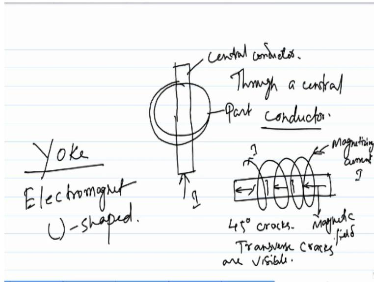
The other method is, to use an induced field, as I mentioned before. So, if you have a circular part and you need to magnetize this to inspect the circumference then, what you can do, you can have a central conductor carrying the current. So, you can pass the current through a central conductor. So, this will carry the current and induce the field in this part, through this central conductor.
