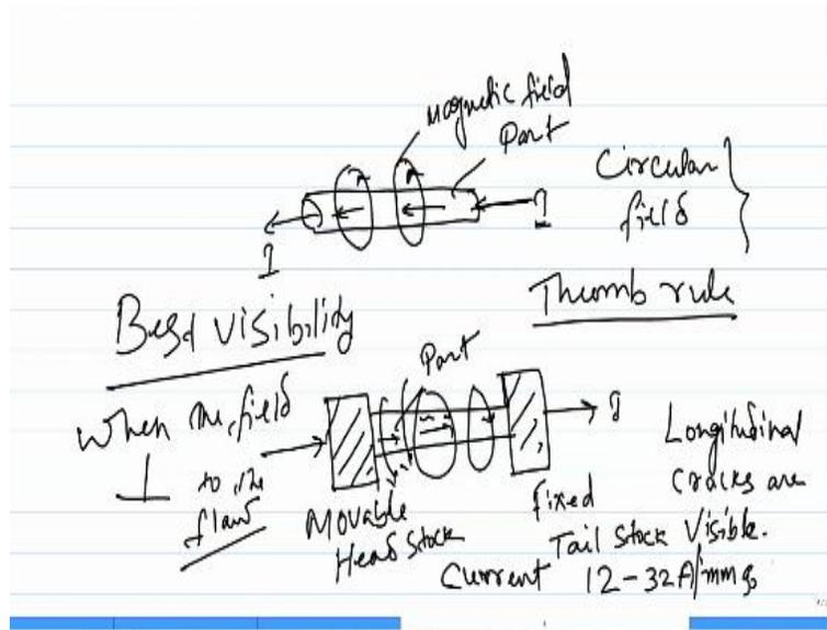
So, in the first case of using this head stock and tail stock, so, you could realize that in this case the best visibility, because this is the direction of the field, so, in this case, your cracks which are longitudinal or perpendicular to the field will have the best visibility. And for this case, the magnetic current levels, that one has to use, it depends on the size of the part, in the range of 12 to 32 amps per millimeter of part diameter.
