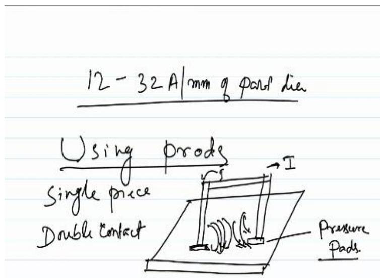
So, if you are using two electrodes as head stock and tail stock then. this is the level of current that you need. Then, you can also use, what is known as prods. So, these are primarily electrodes connected to a power source and when you make a contact of this electrode with the part being examined, it will send the current through the part. So, it could either be a single piece. Let us say, this is the part you have.
