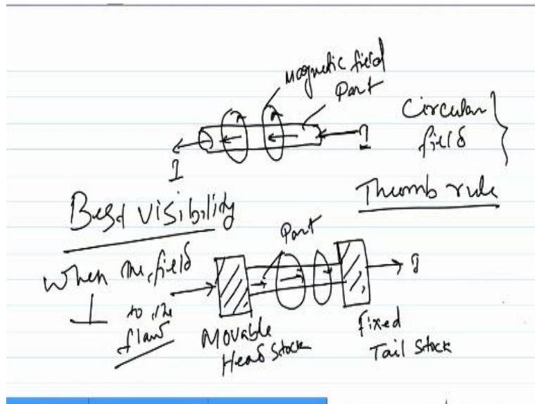
So, let us say, you are using a contact method, so, in that case, the magnetizing current will directly pass through the part. So, that means you need to connect the part in between two electrodes and then switch on the magnetic current and it will magnetize the part. So, let us say, you have a part and this is the current that you are passing through it. So, in this case, if you pass the current in this particular direction, then the magnetic field will be like this.
