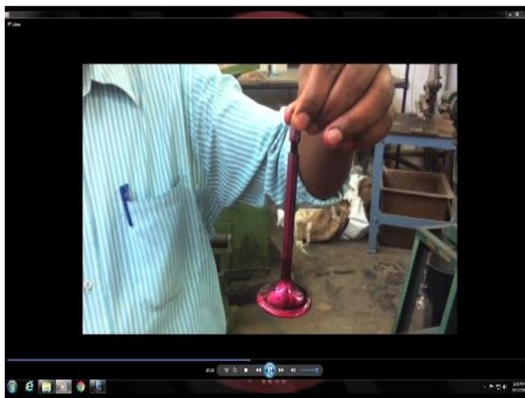
So, here let me first tell you what part we have that we are going to examine. So, if you see this part, this is an automotive exhaust valve, which is used in the engine. So, what he is doing right now, he is cleaning the surface, as I have told you, the first step of the process to clean the
