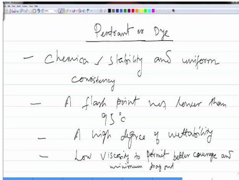
So, the first characteristics or property of this liquid is that, it should be chemically stable and it should also have uniform physical consistency. That means it is not have one density in one part and some other density in the other parts. Then, it should have a flash point, which should not be lower than 95 degree Celsius. So, it is close to 100 degrees that means it is not a flammable liquid. You should be able to handle it properly without the hazards of fire and all that.
