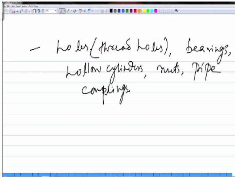
Then, hollow parts or holes. If you have hollow parts, what kind of particles you can apply. You can apply a slurry or magnetic paint kind of thing or a magnetic rubber. So, like, in thread holes, then, other part like bearings, hollow cylinder, nuts and pipe couplings. So, this is some of the applications of magnetic particle testing.
