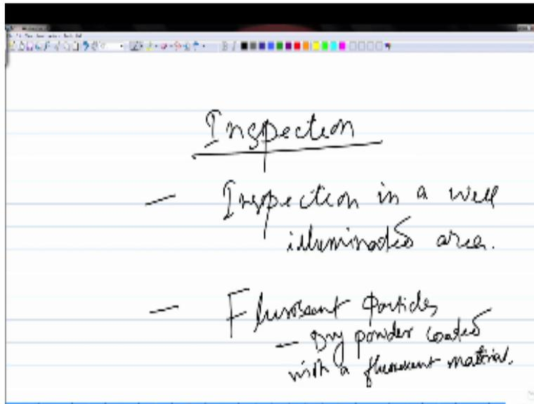
So, in case of dry powder, these powders are many time coated with a color. They can also be coated with a fluorescent material.
