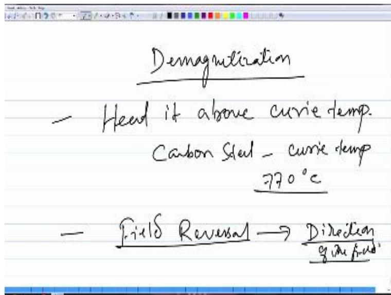
So, there again, knowing the direction of the field helps you. So, this is the another advantage, if you know the direction of the magnetic field. The other advantages, we have already seen, like the orientation of the defects with respect to the direction of the field. The visibility of a defect to depend on that, and the other advantage you have, if you know the direction, is this. So, these are the two methods. These are the two ways by which you can demagnetize the part.
