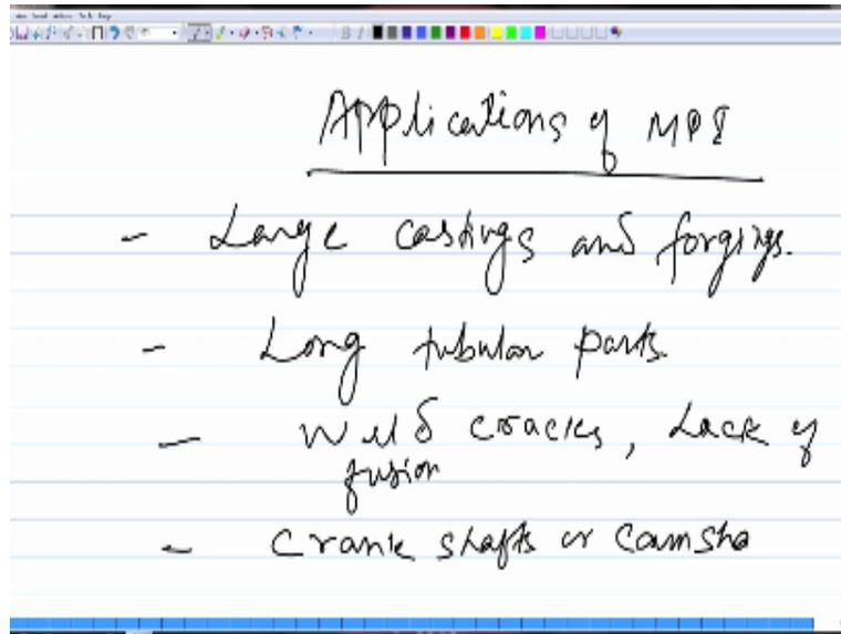
And finally, let us see, what are the applications of magnetic particle testing. So, this can be applied for large castings and forgings for inspecting the surface flaws. It can also be used for long tubular parts, weld cracks, then, in welding, lack of fusion, which is a welding defect that can be inspected, then, parts like crankshafts or camshafts can also be inspected.
