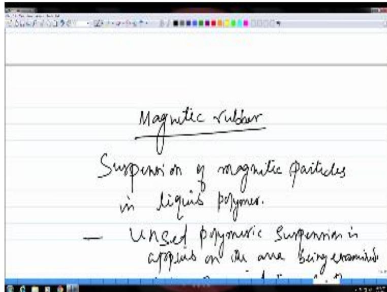
So, we have talked about the magnetizing methods and then, how the particles are applied what kind of particles you have and so on. And we have also seen depending on the condition of the surface or the kind of part you have, you choose different kinds of powder. Either wet suspension and in the wet method itself, we saw there are different kinds of suspensions, depending on what is the part being examined and then depending on the surface condition.
