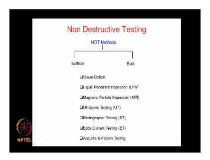
So if you want to examine which is lying beneath, you need to come back to these NDT methods, that is where lies the utility of the NDT methods, where you can apply a particular NDT method to visualize and get visible indication of deflects and flaws which are not visible to the naked eye. So, that's the purpose of this particular course to see how exactly a particular
