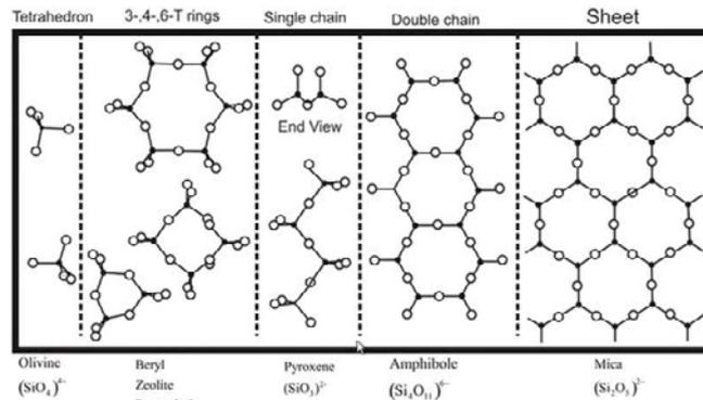
Fig. : Arranging  $\text{SiO}_4$  tetrahedra in different silicates. The Exception is the sheet that extends indefinitely in all Directions in the plane.
