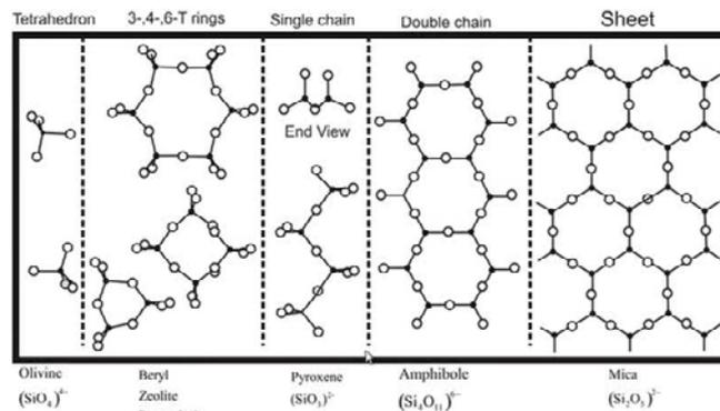
Fig. : Arranging SiO<sub>4</sub> tetrahedra in different silicates. The Exception is the sheet that extends indefinitely in all Directions in the plane.
