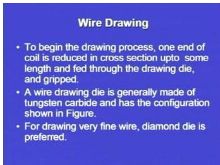
To begin the drawing process, how wire drawing is done? To begin the drawing process, one end of the coil is reduced in cross section up to some length, and fed through the drawing die and gripped. So, how the operation actually is performed, we have seen in one of the previous diagrams that the wire is coming from the coil, and it is getting submerged into the or immersed into the lubricant then it enters into the die cavity, and it is pulled by the draw block that is a very basic diagram.
