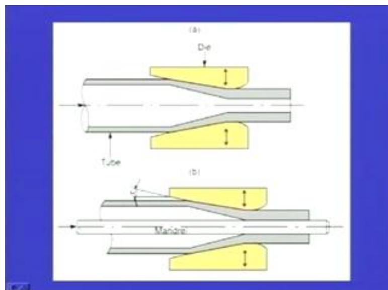
So, now this diagram briefly explains the principle of swaging, though this is not a very complete diagram. We can see that the die has been shown, this is the die which is there, this yellow colored portion is the die portion, and this is the tube that is being swaged. So, we can see this is coming from this direction, and going out from this direction. So, what is the basic cross section of a die? That we will see in a subsequent slide.
