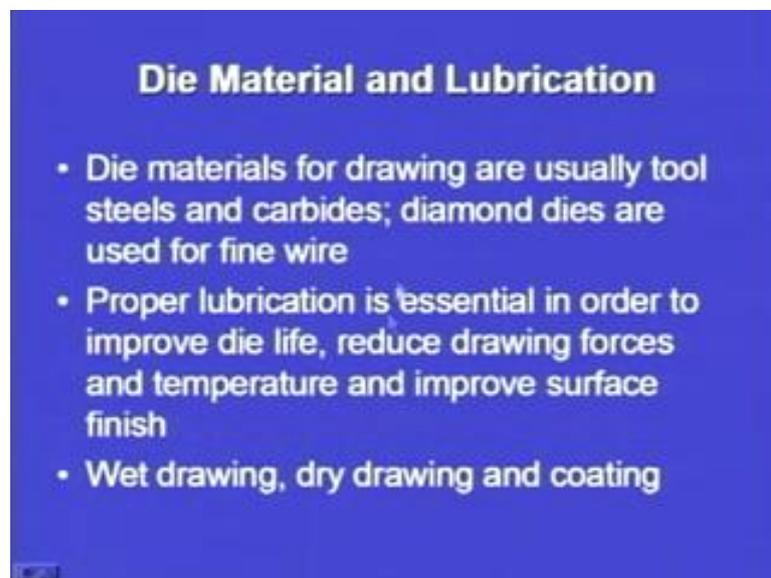
Now, coming on to the die material and lubrication, we have seen that the die, what is the cross section of the die? What are the different angles that are given to the die? How the die is labeled? What are the different portions of the die? There is an approach angle; there is a relief angle towards the end. Then there is a land, different portions have been shown, but the material of the die is also very, very important. Then the weather should
