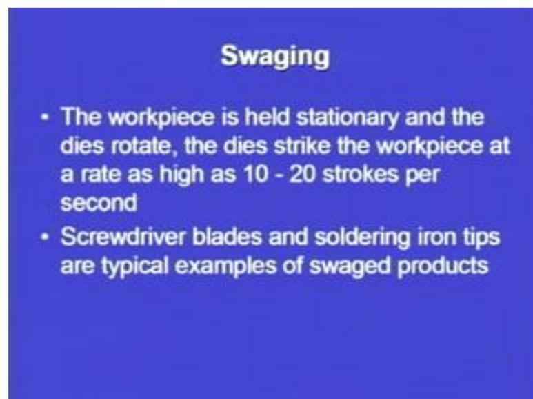
In case of swaging, the work piece is held stationary and the dies will rotate. Already in the brief introduction of swaging process, we have discussed that the dies in this case are rotating in a circular fashion. The dies strike the work piece at the rate as high as 10 to 20 strokes per second. So, we can see that per second we can have 20 strokes. So, the
