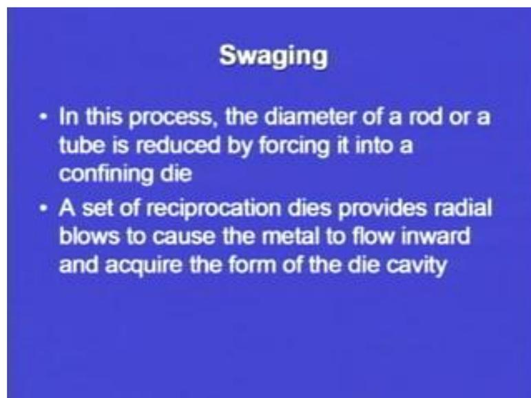
Now swaging, the basic principle of swaging is that in this process, the diameter of the rod or a tube is reduced by forcing it into a confining die. So, confining die will have the dimension, according to the final dimension of the rod or the tube that we want. If we want to make use of a tube, we will make use of a mandrel in that process. So, basically swaging is a process in which the diameter of the rod or a tube will be reduced by a forcing it through a die.
