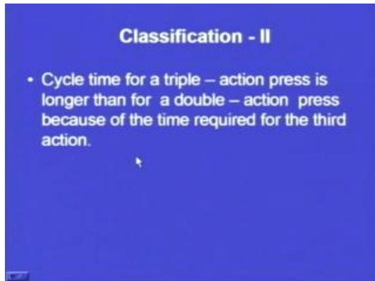
Cycle time for a triple action press is longer than for a double action press because of the time required for the third action. So, this is quite normal that when we have to perform another operation, so the cycle time that will add on the complete cycle time, the cycle time or that amount of time that is required using a triple action press is more than a double action press. Coming on to the third important classification that is on the basis of frame and construction.
