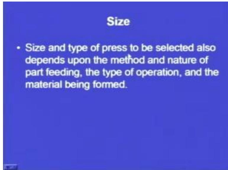
Also, the size and type of press to be selected depends upon method and nature of part feeding, the type of operation and the material being formed. So, on these three parameters also, size and type of press will depend. What are those? These three parameters, this is a nature of the part feeding, the type of operation and the material being formed.
