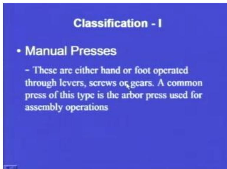
Now, what is the manual press or what are the different manual presses? Now, manual presses are either hand or foot operated through levers, screws or gears. So, manual as
