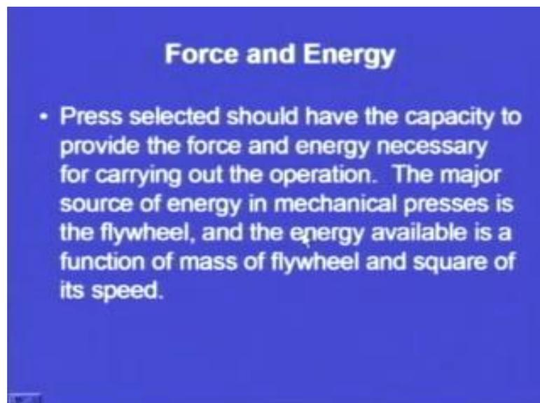
Now, force and energy requirements. This is another important parameter of acting the selection of a press. Press selected should have the capacity to provide the force, and
