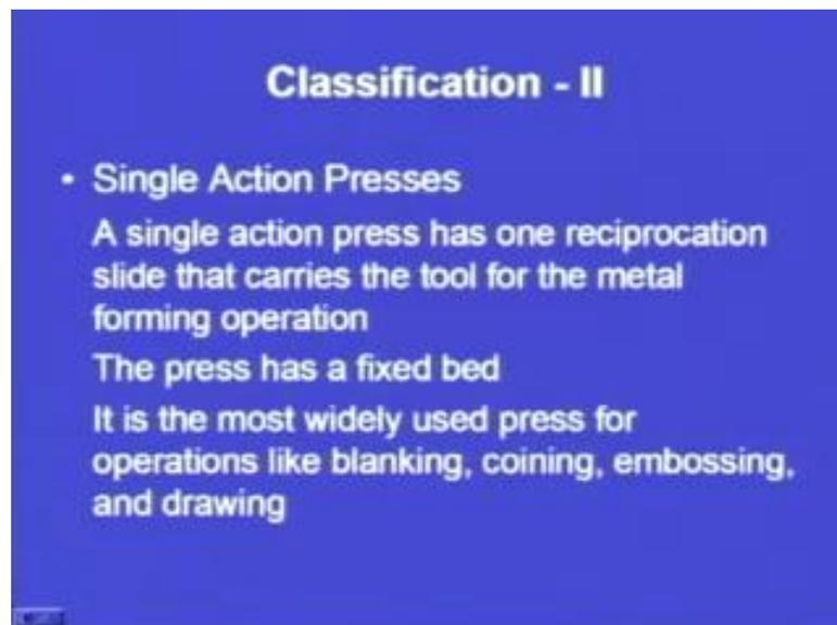
Coming on to the single action presses. A single action press has one reciprocating slide that carries the tool for the metal forming operation. So, it has only one reciprocating slide that is carrying the tool. The tool sometimes is the punch in the die set. So, the
