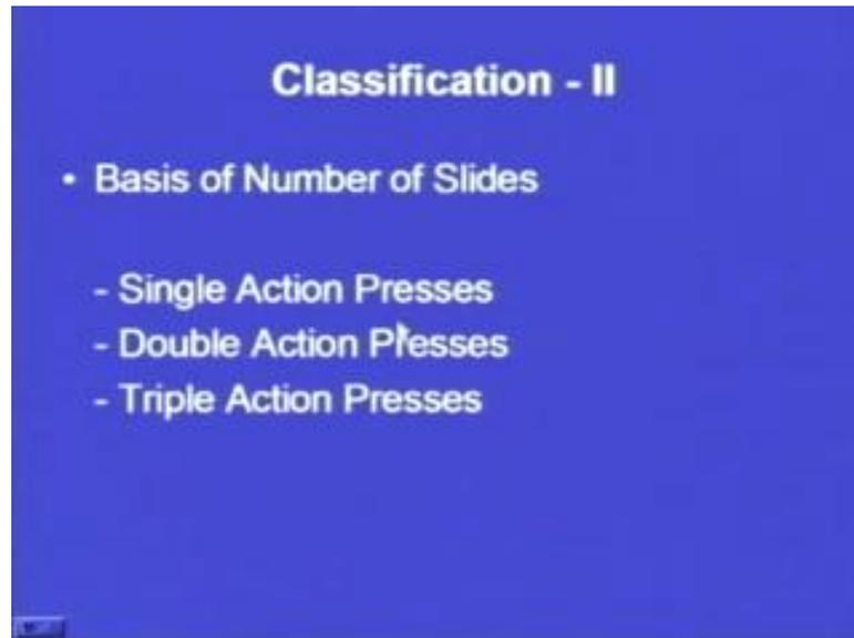
Now, first classification was on the basis of sources of power. Now, the second classification is on the basis of number of slides. Now, on the basis of number of slides, we can have three basic types of presses. These three basic type presses are: Single action presses, double action presses and triple action presses.
