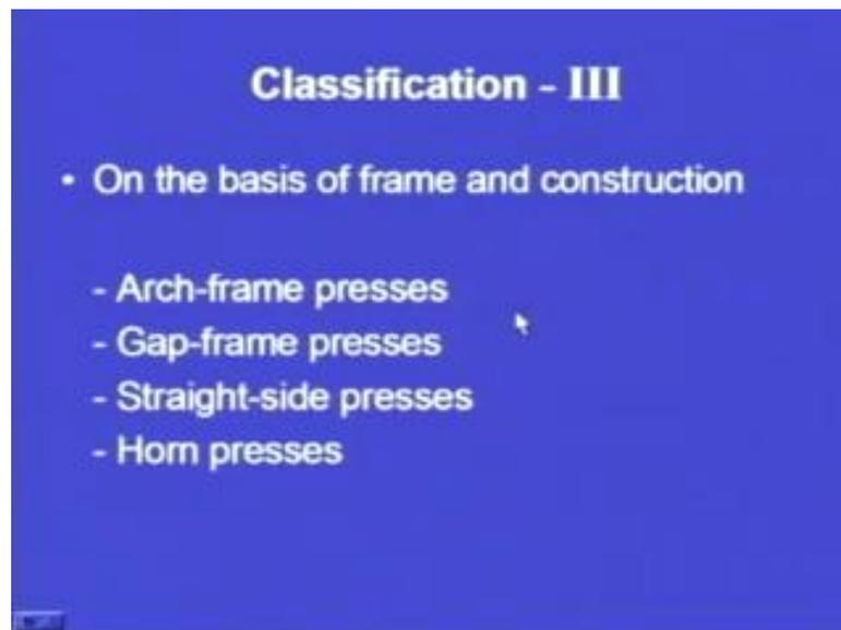
So, on the basis of frame and construction, we can have different types of presses. What are those different types of presses? There are arch-frame presses, gap frame presses, straight side presses and horn presses. So, we will try to understand these different types of presses with the help of a very simple diagram.
