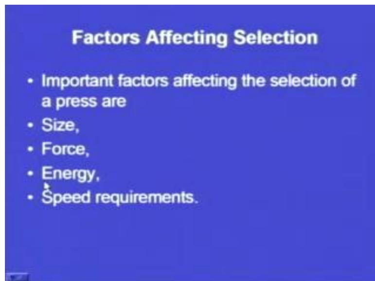
Now, the different factors, which help us to select a process. What are the various factors that have to be taken into consideration? So, important factors affecting the selection of a press, these are size force energy and speed requirement. So, force and energy can be clubbed together as one of the specifications, or one of the parameters affecting the selection of the press. So, we have size force and energy and speed requirements.
