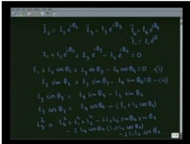
To analyze this equation, we write,  $\bar{l}_2$  in terms of complex exponential notation, that is  $l_2 e^{i\theta_2}$ . Same, for  $\bar{l}_3 = l_3 e^{i\theta_3}$  and  $\bar{l}_4 = l_4 e^{i\theta_4}$ . Since  $\theta_1$  is zero, the  $\bar{l}_1$  is simply,  $l_1 e^{i \cdot 0} = 1$ . So, the loop closure equation, let us substitute these complex exponential notation, so you get,
