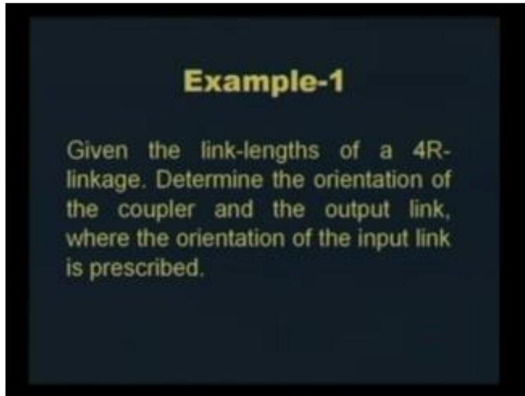
So, we start with an example that is the simplest one. Suppose, we are given all the link-lengths of a 4R-linkage, then determine the orientation of the coupler and the output link, when the orientation of the input link is prescribed. This is a problem of displacement analysis. We are given all the kinematic dimensions and the position of the input link and the task is to determine the position of all other moving links for that particular configuration.
