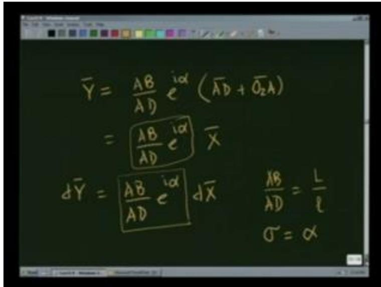
So you see that the position of these two vectors, that is the point E and the point D is given by point  $\overline{Y}$  and  $\overline{X}$  and they are related through this equation.  $\overline{Y}$  is changing with time,  $\overline{X}$  is changing with time but the link lengths AB, AD and the angle  $\alpha$  of that triangle are not changing with time. So, these factors are constants i.e., independent of time. So, movement of the point  $d\overline{Y}$  can be written as,
