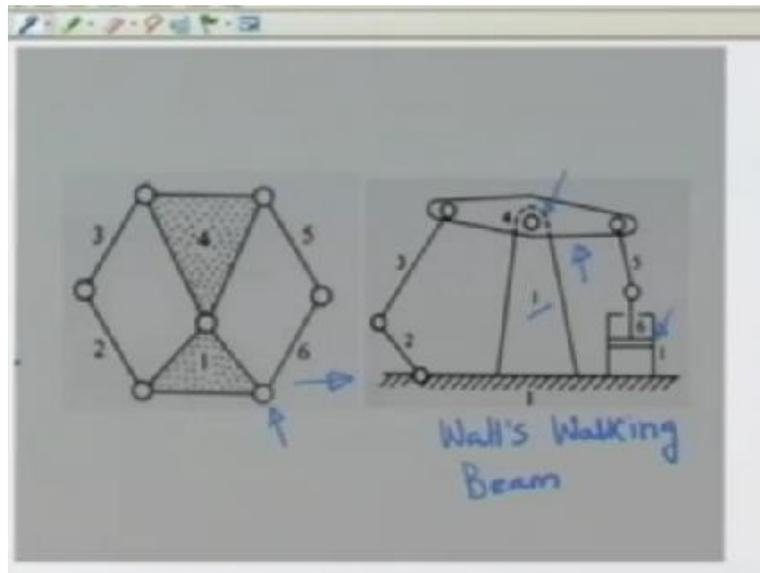
An example of another type of possible Watt's mechanism let us consider above figure. Here as we started from a Watt's chain which has two ternary links 1 and 4 and 4 binary
