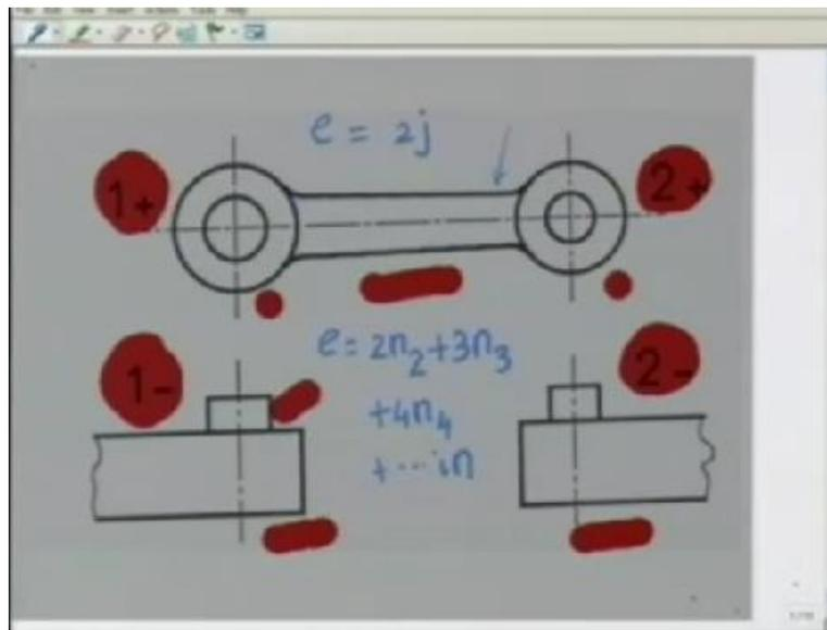
In this figure, we see there is one link which is connected to two other links through the revolute pairs here and here. To note that at each of these revolute pairs we have two elements, say 1- which is the pin which goes into the hole which is denoted by 1+. So this 1+ and 1-, we shall call elements, thus at each revolute pair we have two elements. Similarly, the two elements at the other revolute pairs are 2+ and 2-.
