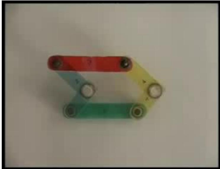
Let us now look at the model of above parallelogram linkage with a redundant coupler. As we see these 2 links are extended at  $90^\circ$  and there are 2 parallel couplers. Consequently, here we shall be able to maintain the parallelogram configuration throughout the cycle of motion. It can never flip back into anti-parallelogram configuration.
