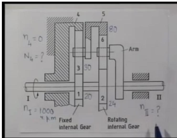
Let me now solve this example of an epicyclic gear train. This is an epicyclic gear train, where the input shaft 1 is connected to this compound gear 1 and 2, that is the speed of this shaft is the same as that of speed of gear 1 and gear 2. Gear 1 is connected to this planet gear, gear 3. Gear 3 is carried by this arm that means there is a revolute pair hear
