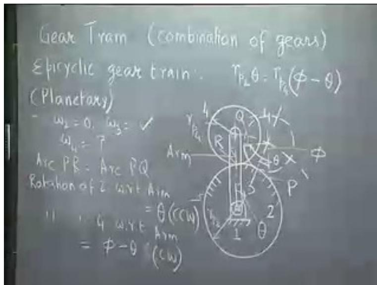
Towards that, we want to study the relative motion between 2, 3 and 4 and as I said, it has two degrees of freedom, so only two input speeds are necessary to fix the output speed. We say we give input to gear 2 and gear 3 and find what is the speed of gear 4? That means, we prescribe the angular velocity of body 2 and body 3 and we want to find that of body 4. So, we can study this relative motion.
