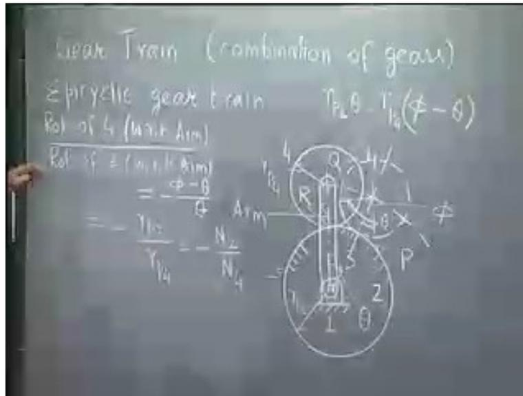
So if we divide this by this, we consider rotation of gear 4 but with respect to arm and rotation of gear 2 again with respect to arm. If I talk of this relative rotation and take the ratio, we are getting  $\phi - \theta$  that is in the clockwise direction, divided by  $\theta$  that is in the counter-clockwise direction. So I put a negative sign.
