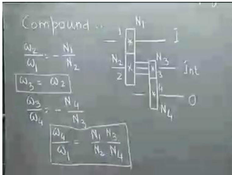
Now, let me discuss how to analyze compound gear train? Let me now discuss what we mean by a compound gear train. In a compound gear train, there will be more than one gear on some shaft, either on the input shaft or output shaft or intermediate shaft, there must be one shaft in the gear train where there will be more than one gear on the shaft.
