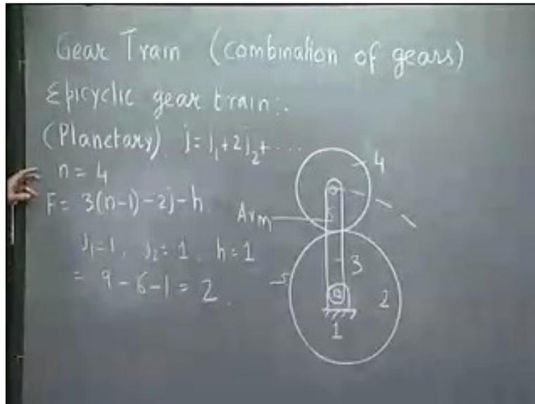
As usual we give them fixed link 1. This gear let me call 2, this arm is 3 and this gear 4. So, this is a 4 linked mechanism, n is 4. First we calculate, the degrees of freedom of this mechanism. Degree of freedom F can be obtained from  $3(n-1) - 2j - h$ , where j is the equivalent number of simple hinges that is,  $j_1 + 2j_2 + \dots$  like that and h is the number of higher pair and n is the total number of links.
