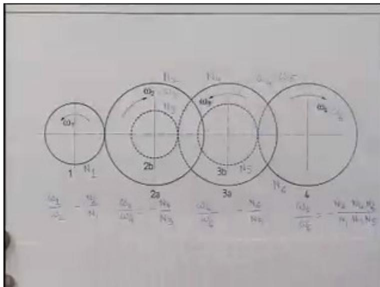
The above figure shows again a compound gear train. As we see, on these two there are two gears, one here and one there. This gear is connected to this gear and on the same shaft there is this gear which connects to this gear and on the same shaft there is another gear which is connected to this gear. From here to here, the speed rotation is being transmitted. These two are intermediate shafts. So, this is a compound gear train.
