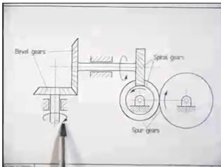
intermediate shaft. Input shaft, output shaft and there is an intermediate shaft, and there is one gear on each shaft and the motion from this input is transmitted to the output. Now, analysis of such a simple gear train is almost trivial. As we see here, these are all external gearing and the number of teeth is say  $N_1$  on this gear,  $N_2$  on this gear and  $N_3$  on this gear.
