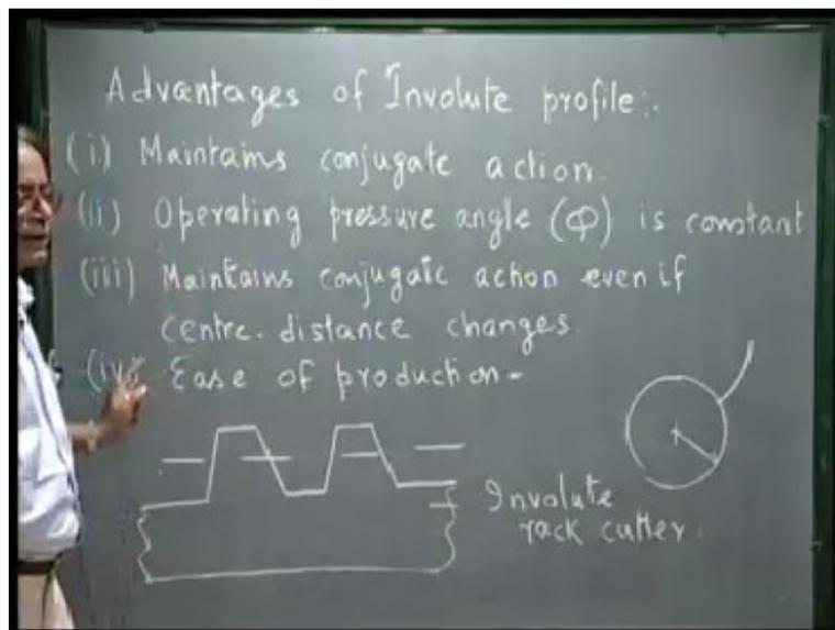
In our last lecture, we have already seen that a pair of involute profiles can maintain the conjugate action. That is, it satisfies the fundamental law of gearing, that is, it maintains constant angular velocity ratio between the two shafts.
