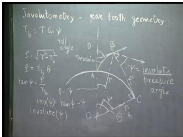
The result that we will obtain from this involutometry will be very useful to determine various proportions of the gear teeth, which are involutes. So we can say application of involutometry in gear tooth geometry. I repeat we will discuss of course only the very basics of this gear tooth geometry. You can always refer to hand book for the details that we may like to know.
