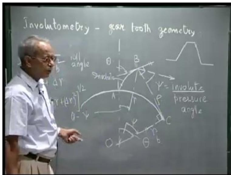
That is what we said that if we have an involute rack, let the tooth profile from the base circle as it come out, it comes out in the form of a straight line. So, the tooth profile of an involute rack is a straight line and which can maintain conjugate action with an involute gear or involute pinion and that gives the advantage that we can use such a rack cutter to generate the involute tooth profile on a circular gear blank.
