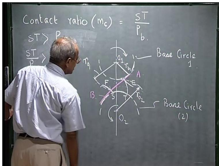
So, to maintain contact all the time between these two pair of gears,  $ST$  must be more than base pitch. And it is this ratio  $ST$  by base pitch, which we have defined by  $P_b$  must be more than 1. We define  $m_c$  as  $ST/P_b$ . What is  $ST$ ? It is the movement of this tooth measured along the base circle from the start to the end of the engagement. To calculate  $m_c$  we proceed as follows.
