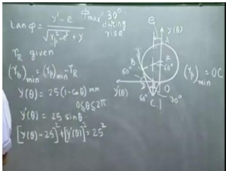
Today, we will take an example to show how from this geometrical construction we can get the optimum values of the prime circle radius and the offset. Of course, the roller radius  $r_R$  is assumed to be given and if I get  $r_p$  the minimum value, then base circle radius minimum  $(r_b)_{\min}$  can get from  $(r_p)_{\min} - r_R$ .
