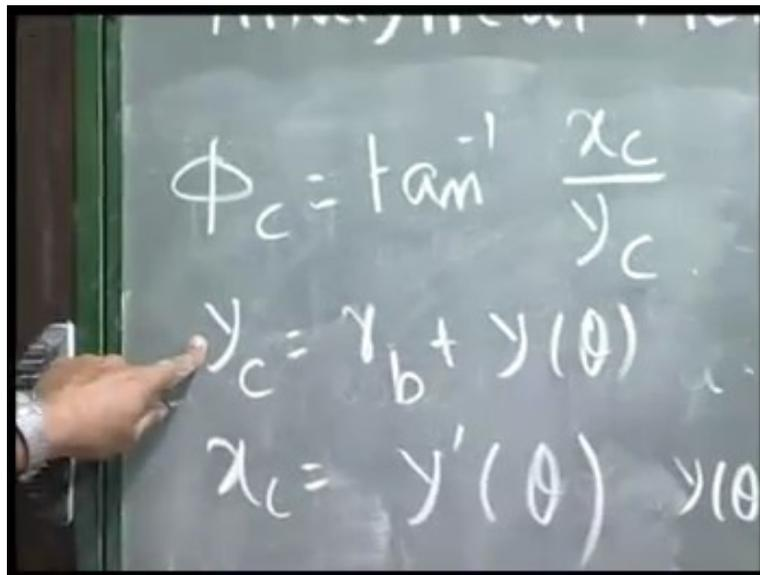
$\phi_c = \tan^{-1} (x_c/y_c)$  and if we remember  $y_c = r_b + y(\theta)$  and  $x_c = y'(\theta)$ . For given  $r_b$  and  $y(\theta)$ , we get  $x_c$ ,  $y_c$  and we get  $\phi_c$  then we can get  $r_c$  and  $\phi_c^{\square}$  and to get the polar coordinate representation of the cam profile with  $O_2$  as the origin. I will continue this same technique for the roller follower.
