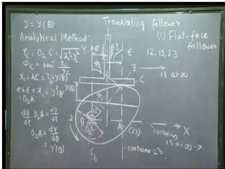
Now that we know how to size the cam, that is how to choose the value of the base circle radius and the proper amount of offset, the next task is to synthesize the cam profile to generate the
