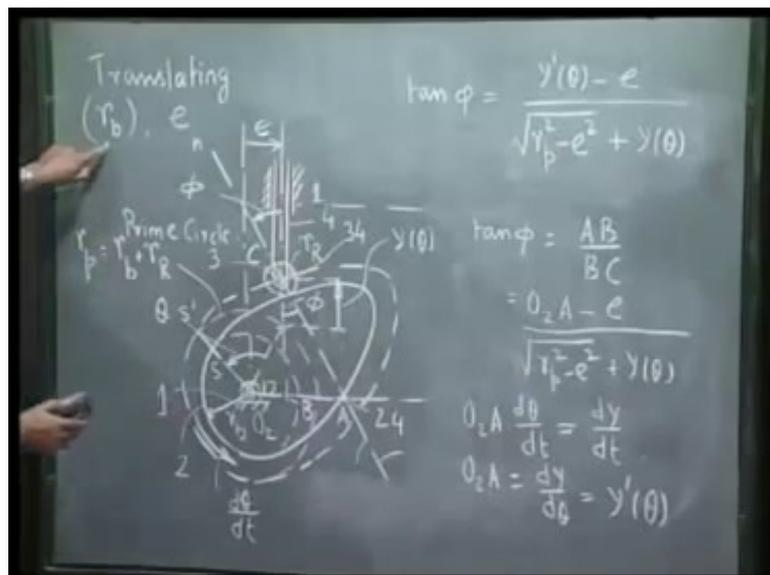
So, what we see that  $\tan \phi$  is AB/BC. If  $\phi$  is the pressure angle, then  $\tan \phi$  is AB/BC, tangent of this angle is AB/BC, where A is at 24 and B is the point of intersection of the guide of the follower with the horizontal line through  $O_2$ , that is line joining  $O_2$  and 24.
