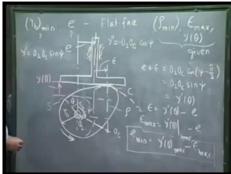
Let us calculate this horizontal distance which is  $e + \epsilon$ ; where  $\epsilon$  is the eccentricity of the driving effort;  $e$  is the offset. It is the distance of the follower axis from the camshaft, that is  $O_2O_C$  cosine of this angle which is  $O_2O_C \cos(\psi - \pi/2)$  which is same as  $O_2O_C \sin \psi$ .
