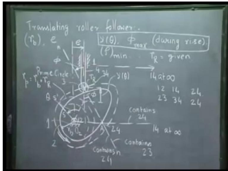
So we are discussing a translating roller follower and we have to determine; what are the optimum values of the base circle radius and the offset that is needed. What are given to us is the desired motion of the follower  $y(\theta)$  and the maximum value of the pressure angle which can be allowed.
