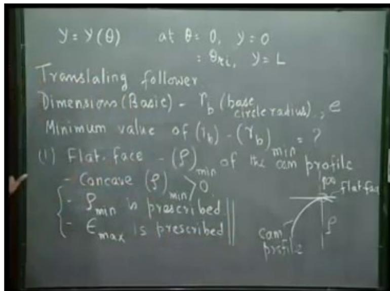
It can be described as a function of the cam rotation  $\theta$ .  $y$ ; the displacement of the trace point as a function of  $\theta$ . This is given to us, that is the desired motion.
