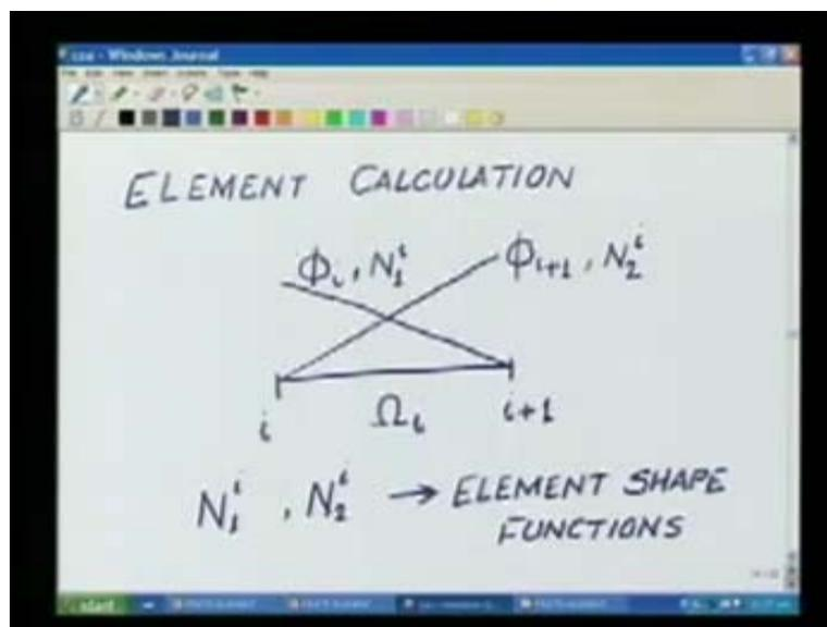
What is the idea? If you take an element  $\omega_i$ , it will have nodes  $i$  and  $i + 1$ . In this element which of the  $\phi_i$ s are going to be non-zero? The  $\phi_i$ s which are going to be non-zero are going to be  $\phi_i$  and  $\phi_{i+1}$ . These  $\phi_i$ s in the element are given a name. The name is  $n_1$  of the element  $i$  and  $n_2$  of the element  $i$ . These  $n_1$  of the element  $i$  and  $n_2$  of the element  $i$  are called Element Shape Functions.
