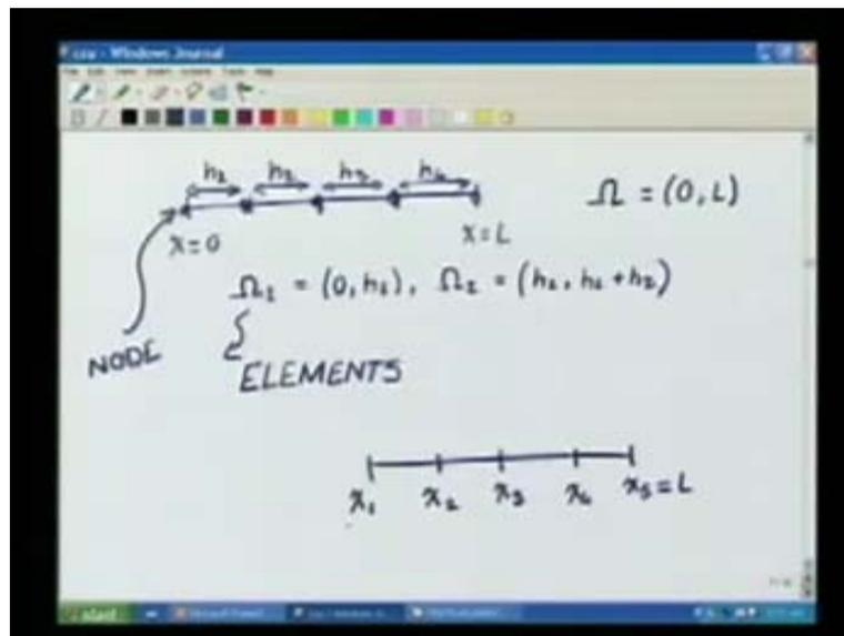
This bar we are going to partition in to smaller pieces by putting these extra points in the domain. These will be I can put them with size  $h_1$  here,  $h_2, h_3$  and  $h_4$  (Refer Slide Time: 17:00).
