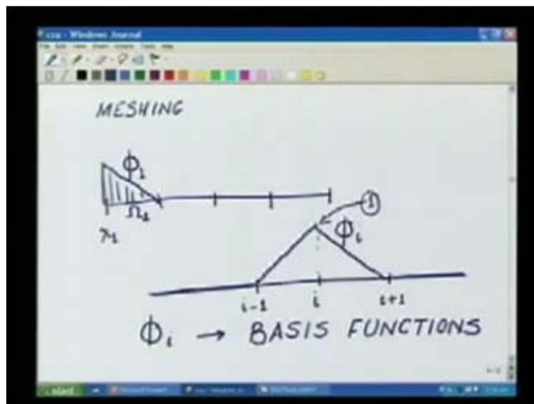
Once I made the mesh, over the nodes I am going to define the functions. How do I define these functions? These functions will be such that; let us take the first node, I will call this function  $\phi_1$  which is linear in the element 1 which is linear in  $\omega_1$  and it has a value 1 at the node 1 and 0 at all other
