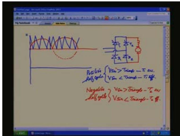
Let us say how we can do it. Let us take our mains wave form. This is the negative side; negative side, we will put it here, rectified mains waveform. This waveform, we will be comparing with a triangle wave, a high frequency triangle wave, high frequency triangle wave, we are doing like this. This frequency of the triangle waveform is high compared to our mains wave. Then, see if you see here, let us take our single phase converter, here  $T_1, T_2$
