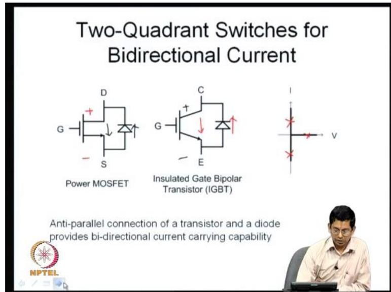
Let us say I have a MOSFET. MOSFET already has a body diode. So, what does it do? You know, once again let me say when it is conducting as I already mentioned it can conduct in this direction, and the diode can conduct in the opposite direction. So, you find that it can conduct in either direction, but how about voltage blocking? It can block voltages with one particular polarity. This is how the way it would be typically connected it will be blocking voltage of this polarity when it is off now.
