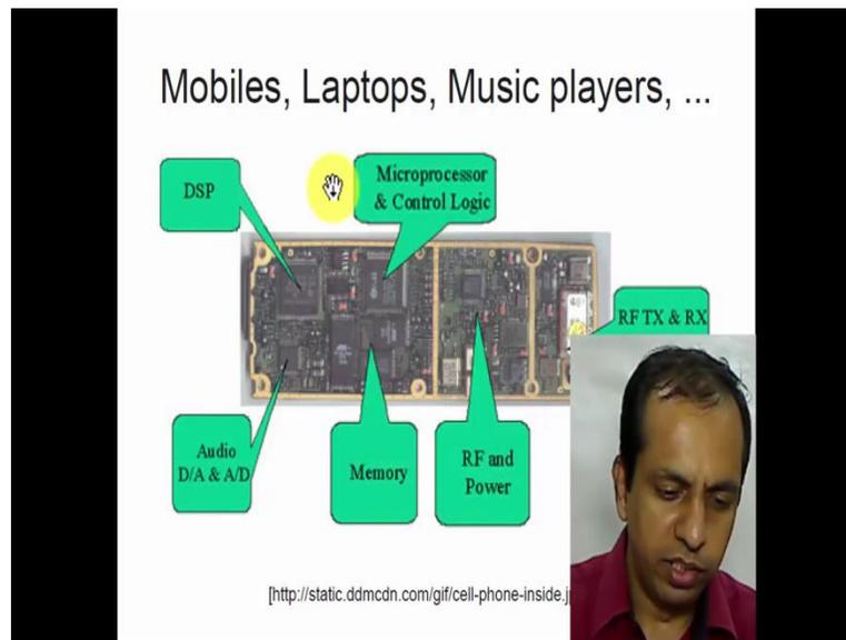
So just to show you an example, I have taken some picture from the web of a mobile phone and it has what are distinctly analog circuits such as audio, digital to analog and analog to digital converters, and RF amplifiers and so on, and RF and power circuits. Also like I said even in digital logic circuits, you need to have an amplifier. So even in memory and microprocessor and control logic and DSP, you will find analog circuits.
