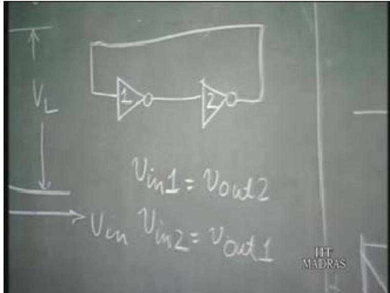
Now suppose you have a circuit like this, you have two inverters we call this inverter one and we call this inverter 2 and so here what you have is you can write  $V_{in1}$  is equal to  $V_{out2}$  and  $V_{in2}$  is equal to  $V_{out1}$ . Now suppose this is the characteristic of inverter one, so I will just remove this, this is the characteristic of an inverter one.
