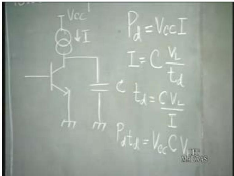
So what is the delay when this capacitance is charged with a current source of value  $i$ ? When you are charging a capacitance  $i$  is equal to  $C \frac{dV}{dt}$ . So if you write  $i$  is equal to  $C$ , so the change in the voltage is  $V_L$  which is the logic swing and the delay will be given
