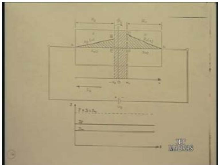
In fact the reason is that there is no recombination in the device, very little recombination I should say because the length of the device is very much smaller compared to the diffusion length and almost all the recombination takes place only at the contact.
