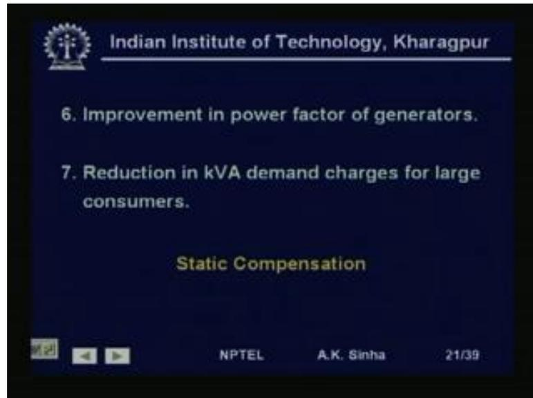
It also helps, as I said if we increase the power factor. It helps the generator also, because it will have to generate, less amount of reactive. Power, which means, that the excitation system, will be working with lesser current. We do not have to over excite, the generators. Of course, for the consumers the advantage is, that is going to be reduction in their k V A demand charge.
