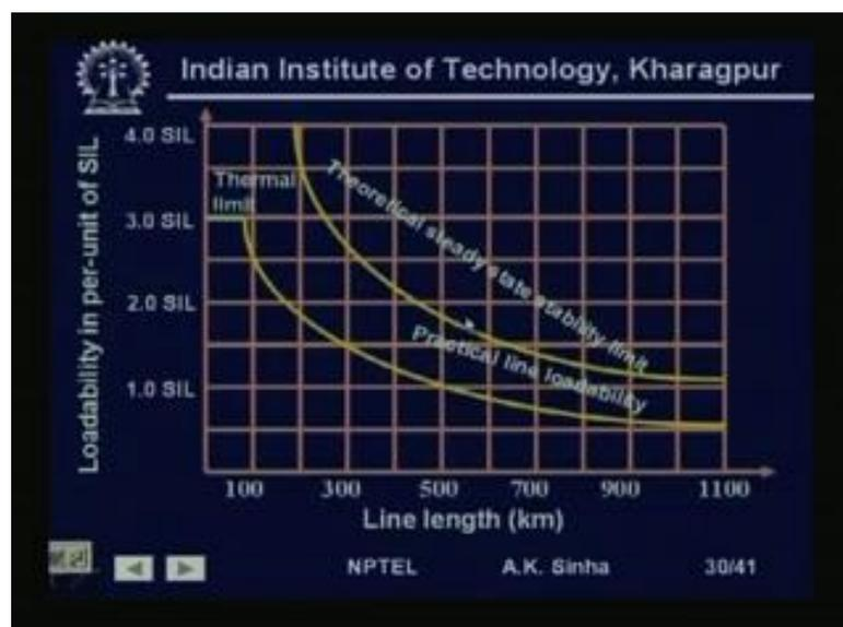
And if we plot this curve, we will get this curve like this, this is the theoretical one, where as the practical one will be much lower, because we normally work at an angle of delta around 30, 35 degrees only not beyond that. Normally between 20 to 30 degrees. And here we see that for short lines, that is lines up to 80 kilo meters also, it is the thermal limit which is the limiting factor for the transmission line load ability.
