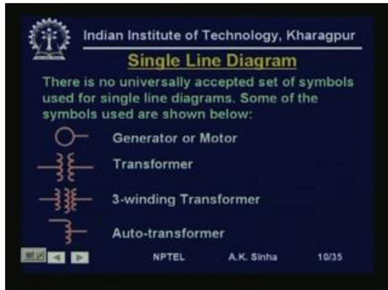
But, we use certain symbols which are more or less. Universal in the sense, that most of the people use these kinds of symbols. Generators is represented like this. Similarly, transformers 2-winding transformers are represented with 2-windings, shown 3-winding transformers. With 3-windings like this and auto transformers are shown in this fashion.
