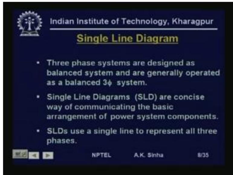
We know that 3 phase systems are designed as balance system. And are generally operated as a balanced 3 phase system, which means that all the equipment which are the 3 phase equipment like generators, motors, transformers. All are designed to be balanced system means. All the 3 phases have equal impedances have the same voltage levels and so on.
