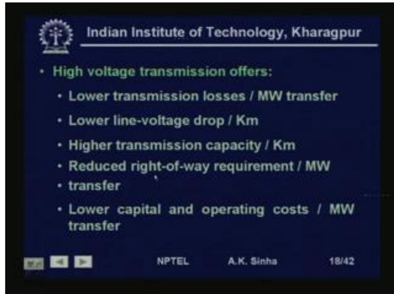
Now, what are the advantages of using high voltage transmission system. First is we have lower transmission losses per megawatt of power being transferred. We have lower line to voltage drop per kilometer. Because, we are working at high voltage the  $i^2 r$  losses. Since the voltage is high, the current will be low for the same amount of power. So,  $i^2 r$  losses are going to be low. So, transmission losses are going to be low, if we work at high voltage.
