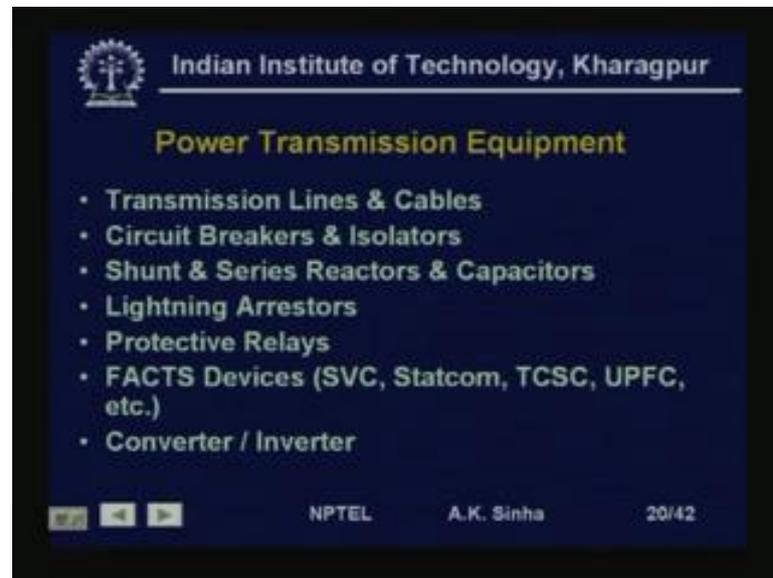
The other equipment that we use are of course, lines and cables to carry the power, circuit breakers and isolators. Circuit breakers are used to disconnect the line when case of falters. Some other reason, isolators are also same kind of switches. That main difference between circuit breakers and isolators are that circuit breakers can break a circuit in which current is flowing. Whereas, isolators are used only to isolate circuit, when it is not carrying any current.
