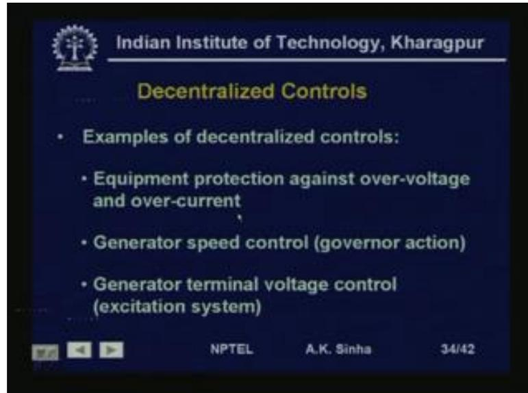
All these are generally done on for centralized control purposes. Whereas, decentralized control as we said speed governing system, protection system, voltage control system. Automatic voltage regulators or the excitation control of each generator, these are decentralized control options.
