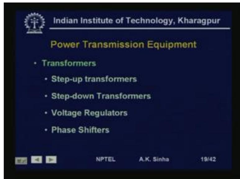
Now, what are the various equipments used in transmission systems. We have step up transformers, as we have already seen. The power is generated at somewhat lower voltage between 11 to 30 KV. We need to step it up to a much higher voltage for transmitting this power. So, we need step up transformers, again at a load end we need to reduce this voltage, because the consumption will be at much lower voltage.
