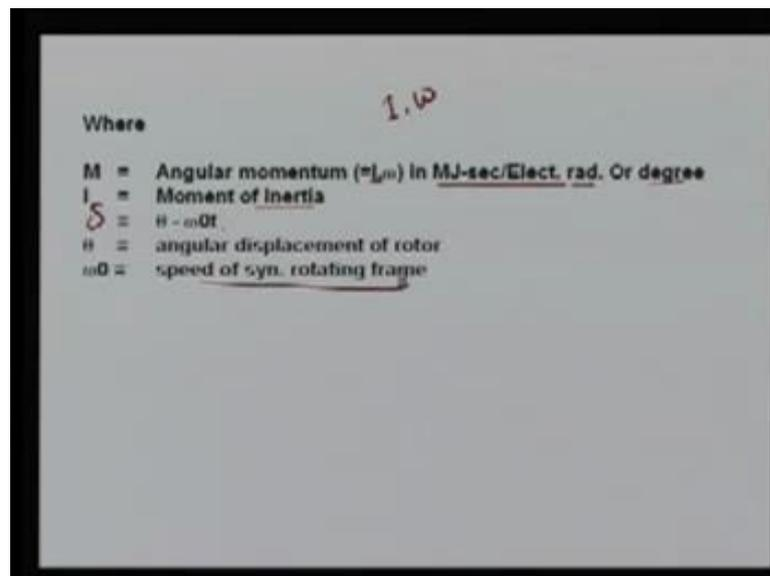
So, this M is angular momentum, and this is defined as inertia i of whole system multiplied by angular speed, and its unit is your mega joule second per electrical radian or degree. i is your moment of inertia, here you  $\delta = \theta - \omega_0 t$ , and theta is angular displacement of rotor, and  $\omega_0$  is the speed of the synchronous rotating frame.
