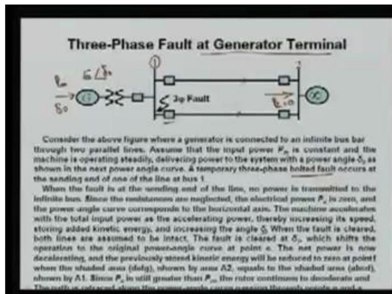
Now, let us see another consideration; means how this equal area criteria, can be useful for determining the other stability criteria. Let us suppose there is some fault. So, if we consider the three phase fault; the three phase fault can be a bus fault, it can be in the line fault, and it can be anywhere in the line either in sending end or in receiving end or in
