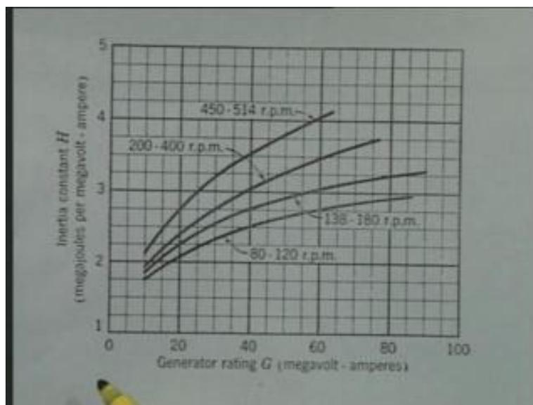
Now this graphs shows the characteristic value of inertia constant  $H$  for a hydro generator. Again on the x axis, we have marked the rating of the machine in MVA and y axis, the inertia constant  $H$  in mega joules per MVA. Here, you see actually that again you find that the machines having different speeds do have different value of inertia constant  $H$ , it increases with increase in the MVA rating of the machine but still you can see actually it lies in a certain range.
