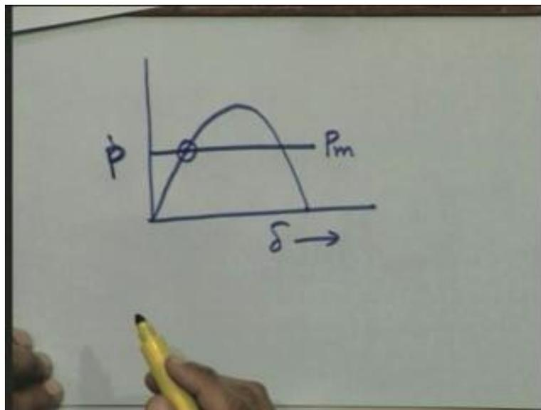
This was your mechanical input line, these are the operating condition and this is the stable operating condition because at this point the slope of the power angle curve is positive. I shall take one small example to find out what is the frequency of oscillations, which we normally come across.
