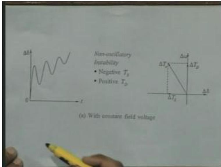
Look here, actually in this diagram the plane is x axis is marked as delta delta y axis is delta omega and in case, the delta T the change in electrical torque lies in the second quadrant then you have 2 components, 1 component is damping torque component, another is the synchronized torque component. Damping torque component is positive while synchronizing torque component comes out to be negative
