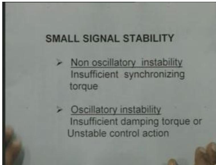
The small signal stability can be classified into 2 categories, one is called non oscillatory instability not a stability instability, it can be non oscillatory instability this occurs because of insufficient synchronizing torque, another is oscillatory instability this is due to insufficient damping torque or by due to unstable control action.
