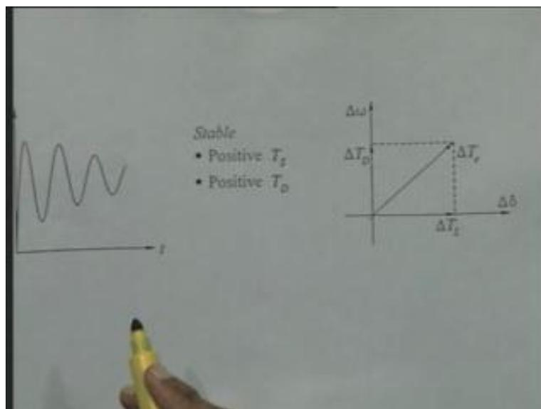
In case  $\Delta T$  lies in the first quadrant of the  $\Delta \delta \Delta \omega$  plane, then both synchronizing torque and damping torques are positive for stability of the system both synchronizing and damping torque should be positive. Okay I will discuss these aspects slight in more detail when we talk about the small signal stability problem.
