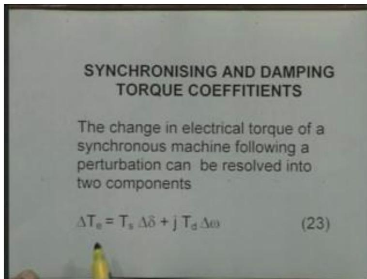
Now we have defined the small signal stability and small signal stability is the ability of the synchronous machines to remain in synchronism under small perturbations. Now when the synchronous machines rotors are oscillating it develops an electrical power  $\Delta T$ , when the rotors are oscillating it produces a electrical torque we call  $\Delta T$ . This torque can be decomposed into two components, one is called synchronizing torque, another is called damping torque.
