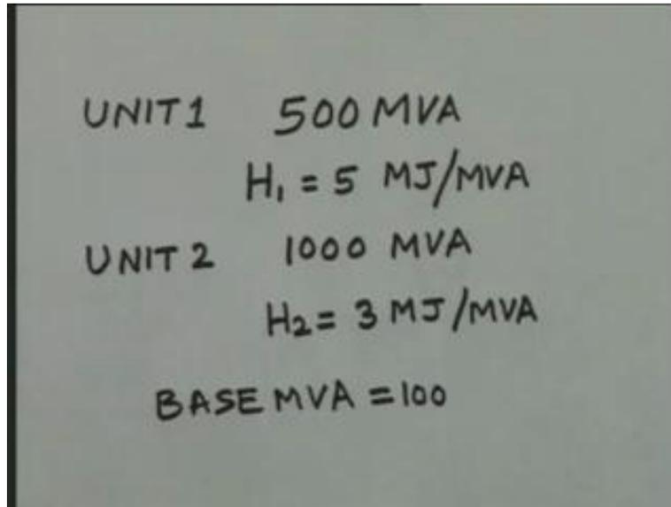
Now just take the example, let us say that unit 1, there are two units are there in the plant, unit 1 is 500 MVA and its inertia constant  $H_1$  is specified as 5 mega joules per MVA, unit 2 1000 MVA its inertia constant say  $H_2$  is 3 mega joules per MVA because the manufacturer provide the information about this H constant on its MVA rating okay.
