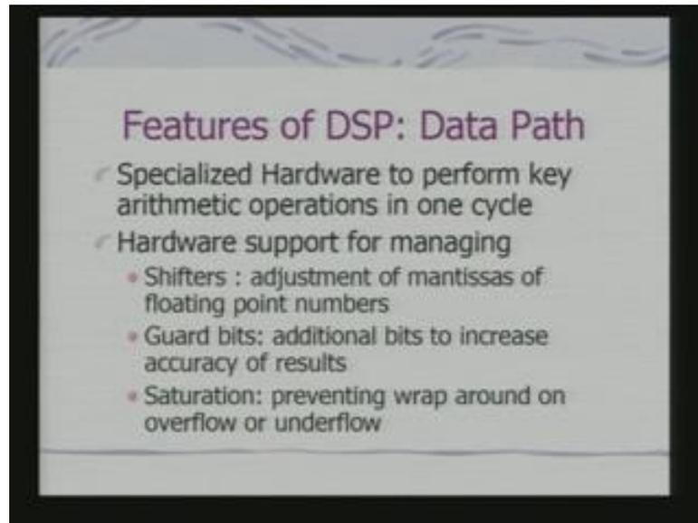
So, let us look at the data path; we have already seen some aspects of the data path and here we are trying to look at some of the other aspects. So, specialized hardware to perform key arithmetic operation in one cycle, and key operation is particularly multiply and multiply accumulate.
