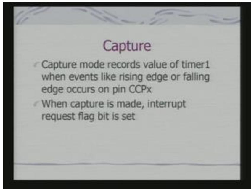
When capture is made what happens, interrupt request flag is set; in fact it can lead to generate, this is one of the source of peripheral interrupt. Now, this is a very interesting feature what you are doing, that you are actually recording events and you are recording events with respect to time. This kind of feature is not commonly available in other processors, okay. You have not found, you have not, must not have encountered them
