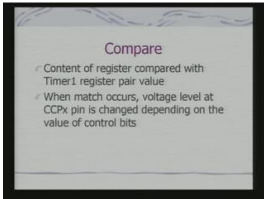
So, the interesting feature here you can realize that you can generate also to this process external signal okay not only just I can possibly match and reset my timer. But not only that I can also generate an external signal to control an external device by taking care of this feature. So, that CCP module in that way is distinct from other kind of peripherals
