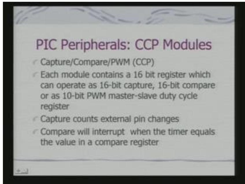
Next, we shall look at another module which is called CCP module- capture, compare, PWM module. There maybe one or more such modules on this PIC micro-controller and this is again targeted for various kinds of control applications. Each of these module contains a 16 bit register which can operate as what we call 16 bit capture register, 16 bit compare register or as 10 bit PWM master-slave duty cycle register. And capture counts
