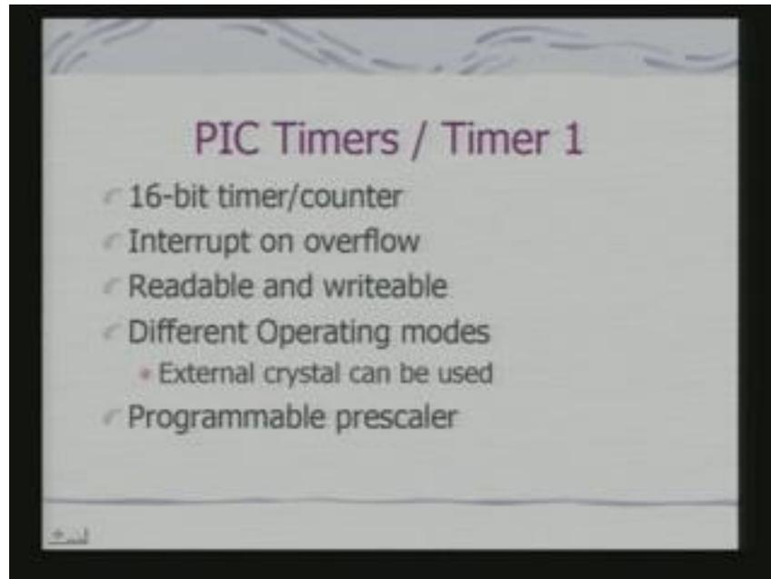
But what is the interesting is, it can operate in different operating modes. It can operate as a synchronized timer, it can operate as a synchronized counter, it can operate as a asynchronous counter. Now, there is a basic difference between them and these differences are interesting. Asynchronous counter, when it works as a synchronized timer, not counter it increments every instruction cycle.
