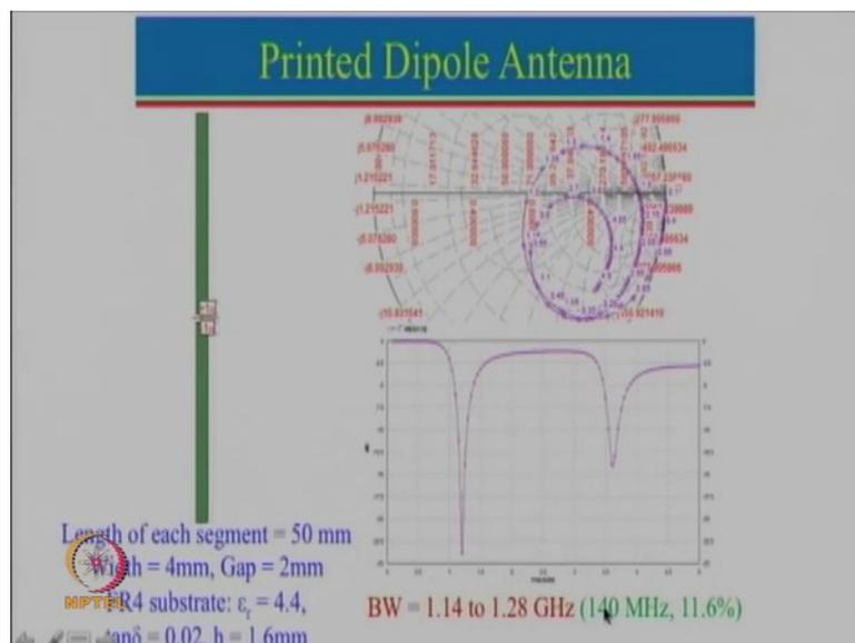
So, here is an example where I have taken an example of a printed dipole antenna, what we have done is we have printed this dipole antenna on a very low cost FR4 substrate this is actually known as also a glass epoxy substrate we use a dielectric constant of 4.4. Typically FR4 substrate dielectric constant may vary from 3.8 up to 4.6. So, this is the substrate which we have. So, 4.4 we took the thickness of the substrate as 1.6 mm.
