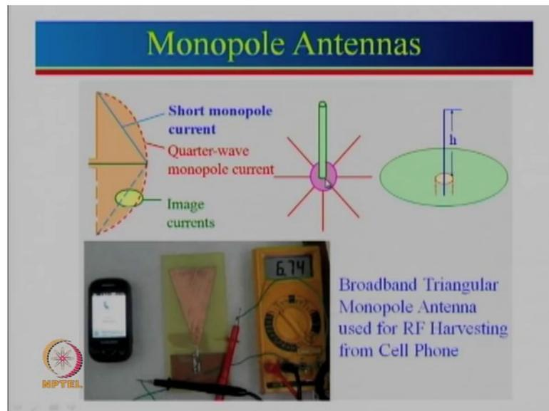
Then let us just look at monopole antenna; monopole antenna is nothing but half of the dipole antenna. So, one can see here this is the complete dipole antenna, but if we just draw the line in between here if we make that plane grounded and then this one is acting as an image, so most of the derivation in the beginning, we will see for infinite ground plane that is for derivation point of view and for infinite ground plane, we can see the image current which is directly there.
