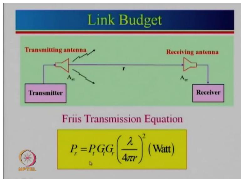
So, let us start with the link budget. A link requires a transmitting antenna, let us say we have a transmitter that transmitter is connected to the transmitting antenna, and then there is a receiver with the receiving antenna, and in between the transmitter and receiver
