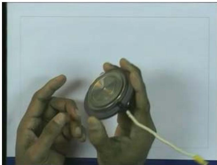
A 600 ampere device, gate terminal and we need to use 2 heat sinks. It is like, formed sandwiched in between 2 heat sinks, a 600 ampere GTO. So, that is about the GTO. So, we have studied SCR, track and GTO.
