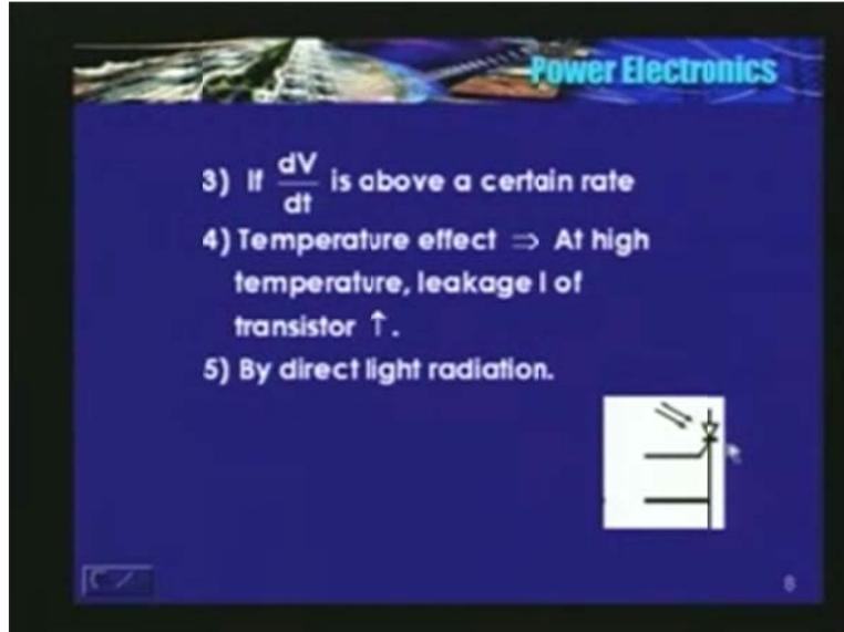
See here, I am radiating light in the junction, to this junction light is being radiated. Definitely, that will increase a junction temperature, leakage currents will increase, they get amplified and thyristor goes into conduction mode. So this method, the last one is used in high voltage applications because as the voltage level increases, it may be difficult to pass the gate current through the conventional wires, lead wires.
