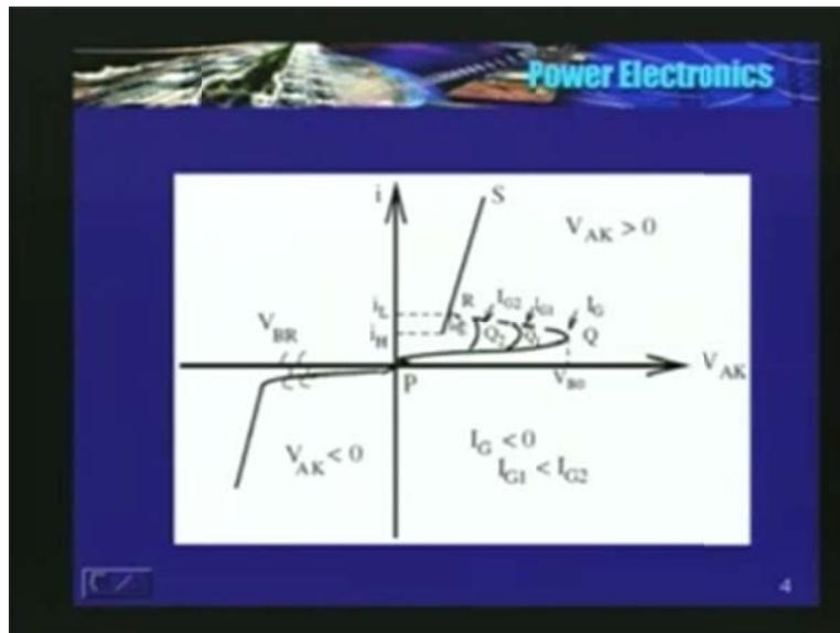
See here, the latching current, this is the latching current,  $I_L$ . Having gone into conduction mode, gate has no control. To turn off the thyristor, the device current should be reduced to a value which is less than the holding current and holding current is always less than the latching current. It is like this, without holding, how can you latch? So, this is the way to remember. Now, what happens if there is a large  $dv$  by  $dt$  across the device?
