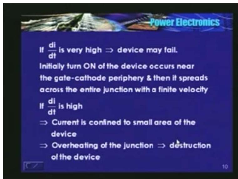
Now, what happens if rate of rise in current is very high? If  $di/dt$  is very high, device may fail. Why it will fail? See, during the initial turn on that occurs, the initial turn on occurs near the gate cathode periphery. Initially the device was blocking, now it starts conducting and it is confined to near gate cathode periphery and it slowly spreads with a finite velocity to the entire junction.
