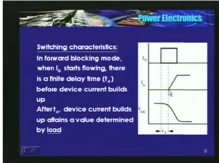
See, there is a finite time, only after which the anode current starts increasing. Again this current, increase in current is determined by the load, this nearby  $dt$  and attains a value given by, not determined by the load. Again here voltage  $V_{AK}$  starts decreasing and attains a very low value which is approximately say 1.5 to 2 volts.
