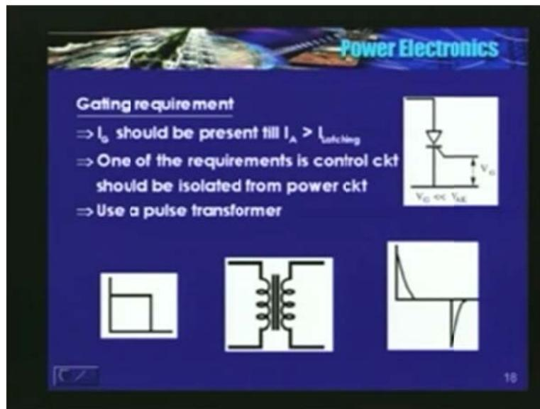
How about the gating requirement? I will just briefly touch up on these issues. Similarly, there are various types of snubbers or protective circuits. Now,  $I_G$  should be present till the anode current is higher than the latching current that is essential. I told you that anode and cathode, they come in series with the load and gate is, gate control element is the gate element, a gate control signal is applied, gate and the cathode terminal. The voltage that is required is very small.
