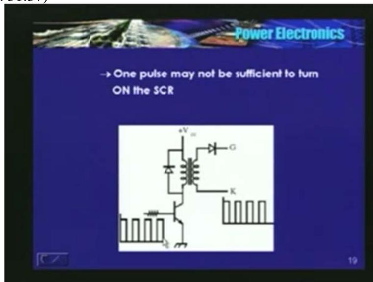
There is a pulse transformer, this pulses are applied to the base of the transistor. These are very narrow pulses, they are very small pulses. So, I am assuming that transformer will not get saturated. So, they are reproduced in the secondary, same pulses. See, transformer is an inductive circuit. Transistor is on during this period and is off during this period. When the transistor is on, current are flowing through the transformer.
