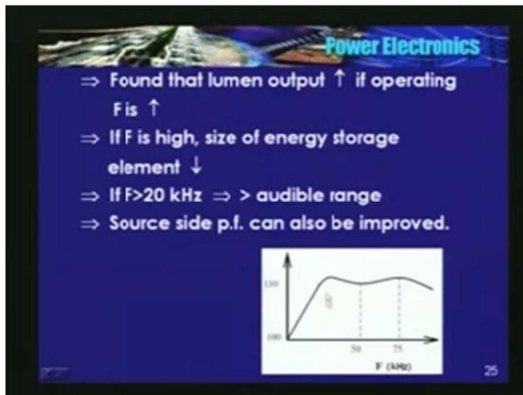
I will just show you the plot of the lumen. This is a lumen output verses the frequency. This frequency is in kilo hertz, not hertz. We have only 50 hertz supply. I have plotted for kilo hertz say, may be 100 at a very low frequency of 50 hertz. 50 hertz, it could be around 100, attains a peak around say, 20 kilo hertz or so. So again, we have a 50 hertz supply and here I need to operate at 20 kilo hertz. Somewhere I need a frequency converter that is about light.
